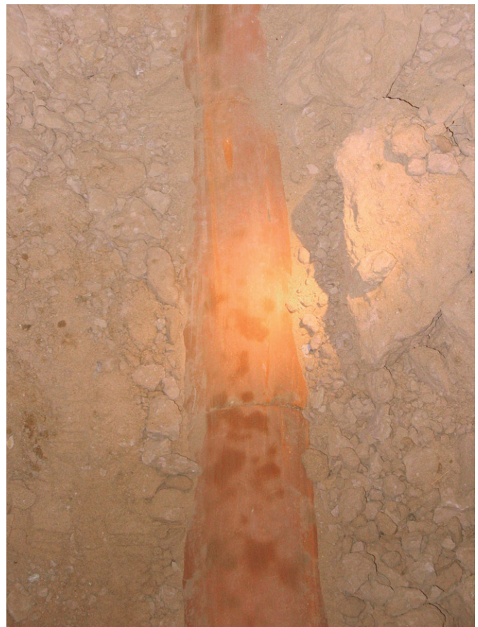
Figure 8. Photographs of the partially exposed clay drainage pipe located west of shot point 2. Left, pipe before shot; right, pipe after shot. Dark spots in right photograph are water stains from spray while the shot geysered. Pipe in photos is approximately 75 cm long (3.5 ft). The diameter of the pipe is 13.5 cm (5.5 in).
