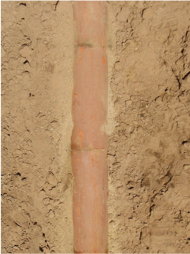
Figure 8. Photographs of the partially exposed clay drainage pipe located west of shot point 2. Left, pipe before shot; right, pipe after shot. Dark spots in right photograph are water stains from spray while the shot geysered. Pipe in photos is approximately 75 cm long (3.5 ft). The diameter of the pipe is 13.5 cm (5.5 in).
