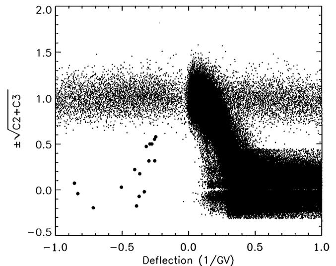
FIG. 2. The signed square root of the absolute value of the  $C2 + C3$  signal vs deflection (proportional to rigidity $^{-1}$ ). The 16 antiprotons have been enhanced (●). Low-mass particles occupy the nearly horizontal band. The Cherenkov counter noise of  $\sim 0.5$  photoelectron can result in negative values. At low amplitude, fluctuations in the signal are exaggerated by the square root. Below 3.2 GeV (0.6 ordinate) the antiprotons are well separated from background.
