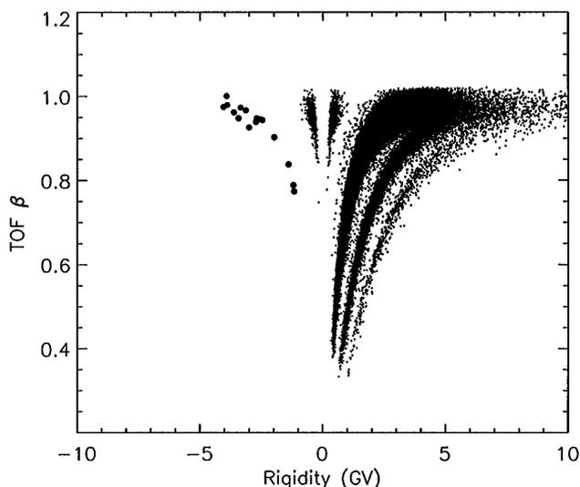
FIG. 1. Velocity determined by the TOF vs rigidity for events with  $C2 + C3 \leq 0.36$ . The 16 antiprotons have been enhanced (●). Protons, deuterium, and tritium are visible at positive rigidity. The protons and antiprotons are clearly separated from the pions, muons, and electrons.
