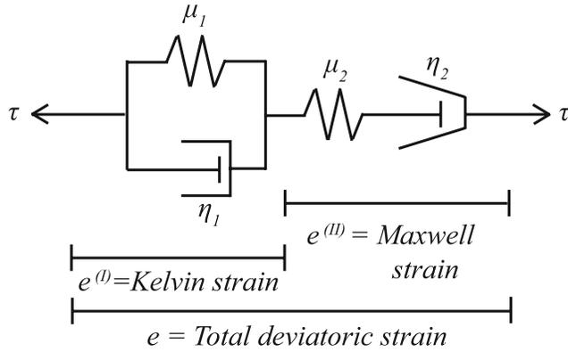
**Figure 2.** Schematic of the nonlinear Burger's body viscoelastic model used for deviatoric stress. The Maxwell viscosity  $\eta_2$  is taken as nonlinear in accordance with Glen's law, and  $e^{(I)}$  is the strain on the Kelvin element.
