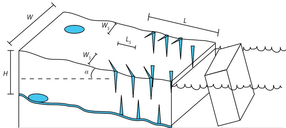
**Figure 1.** Schematic of processes modeled. We model ice deformation modulated by crevassing and fracture, basal processes modulated by hydraulic inputs, and calving of large icebergs. The mass affected has length  $L$ , width  $W$ , and height  $H$ , with ice deformation mostly confined to marginal shear zones and longitudinal deformation zone of size  $W_s$  and  $L_s$ , respectively.
