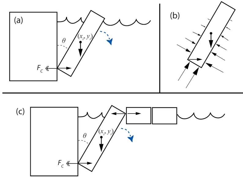
**Figure 6.** (a) Schematic of the tipping iceberg calving process modeled: the dotted arrow schematically denotes the rotation of the iceberg, the double arrow denotes the calving-contact force contributing to the seismic signal, and the solid arrows denote forces. (b) Force vectors acting on the calved iceberg. (c) Schematic of the tipping iceberg with a mechanically competent ice mélange.
