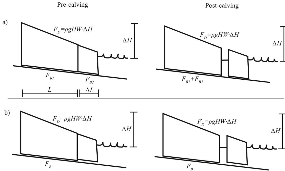
**Figure 4.** Schematic of the forces acting on the glacier precalving and postcalving, (a) with shear resistance on the precalved portion of glacier and (b) without shear resistance. The case shown in Figure 4a can be modeled with lost basal resistance; the case shown in Figure 4b has no net changes in forces.
