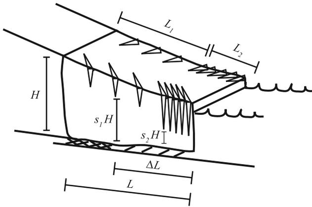
**Figure 3.** Schematic of crevassing and lost basal resistance. Extent of crevassing over length  $L_1$  and  $L_2$  is represented by  $s_1$  and  $s_2$ , respectively. For this case,  $s = (s_1L_1 + s_2L_2)/(L_1 + L_2)$ . Basal resistance is lost over length  $\Delta L$ .
