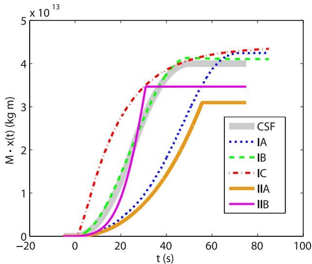
**Figure 8.** Cumulative centroid single force (CSF) amplitude for: the seismic model fitting the observations (CSF), the three variations on the model class I (IA, IB, and IC), and model class II (IIA and IIB). All five model results are consistent with the CSF model used to model seismic observations (see Figure 10).
