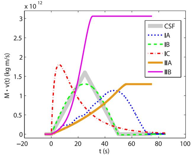
**Figure 9.** CSF rate for: the seismic model fitting the observations (CSF), the three variations on the model class I (IA, IB, and IC), and model class II (IIA and IIB). Model class II does not have a deceleration phase, so the CSF rate does not return to zero. However, the horizontal portion of the curve does not contribute to the CSF amplitude.
