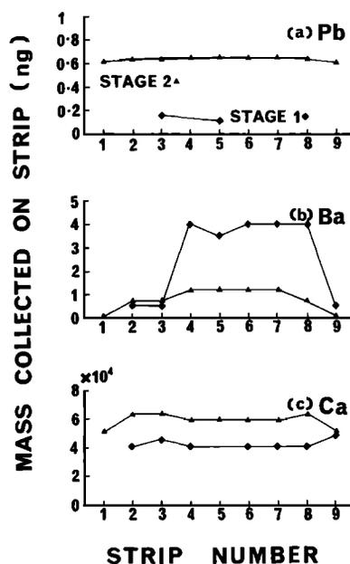
Fig. 1. Distributions of (a) Pb, (b) Ba, and (c) Ca on strips of slotted paper impactor grids placed on the stages 1 and 2 of the cascade impactor.
