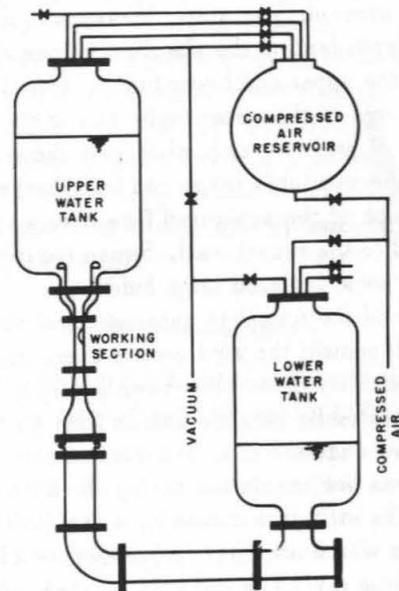
FIG. 1 SCHEMATIC DIAGRAM OF TUNNEL.
