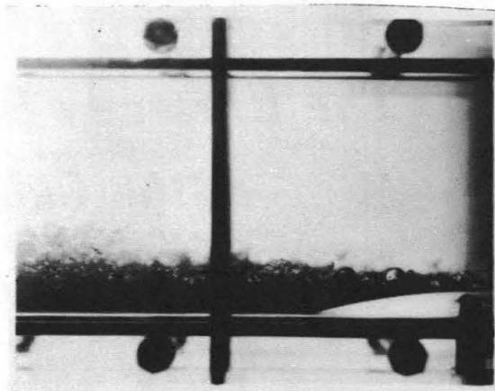
FIG. 3 CAVITATION OCCURRING OVER A CIRCULAR ARC FOIL.
