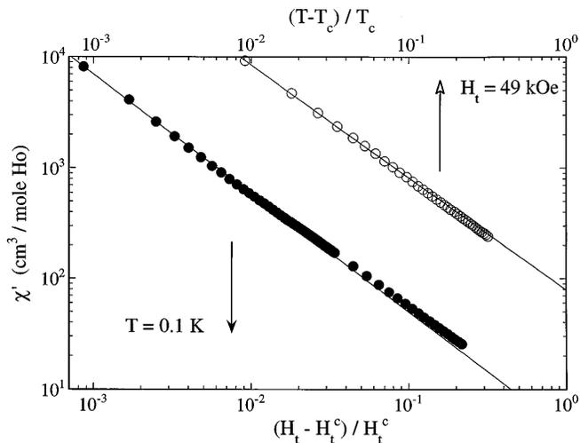
FIG. 2. Mean-field critical behavior of the magnetic susceptibility in the  $T \rightarrow 0$  limit as functions of reduced temperature (open circles,  $T_c = 0.114$  K,  $H_t = 49.0$  kOe) and reduced transverse field (filled circles,  $H_t^c = 49.3$  kOe,  $T = 0.100$  K).
