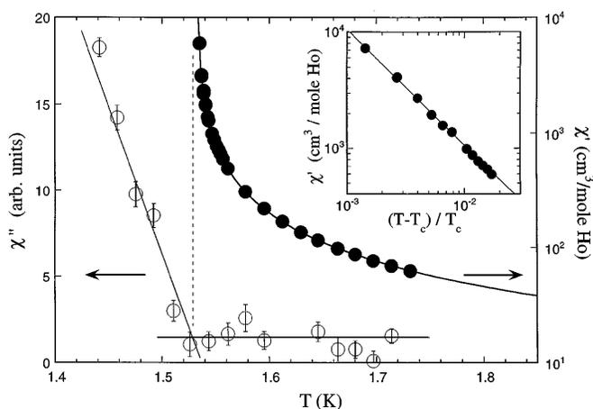
FIG. 1. Divergence of the real part of the magnetic susceptibility (filled circles) and sharp increase in the imaginary part (open circles) at the thermally driven ferromagnetic transition in  $\text{LiHoF}_4$ . Inset: Mean-field critical behavior with  $\chi' \propto t^{-\gamma}$  and best-fit value  $\gamma = 1.00 \pm 0.09$  (line).
