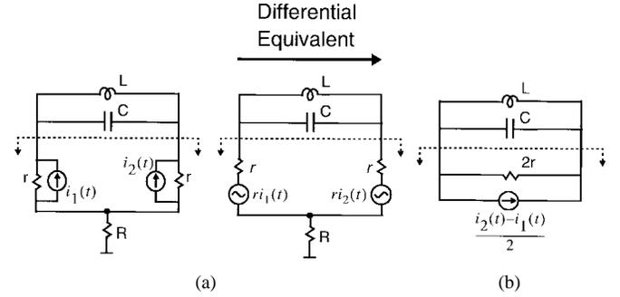
Fig. 6. (a) Simplified model for transistor noise sources. (b) Differential equivalent circuit.
