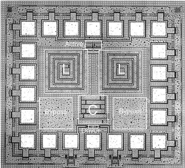
Fig. 11. Die photograph of the differential LC oscillator.
