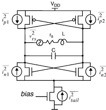
Fig. 5. Complementary LC oscillator with noise sources.
