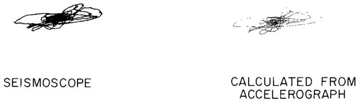
FIG. 2. Computed and measured seismoscope responses. San Fernando earthquake of February 9, 1971.
