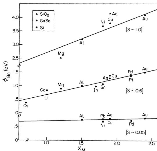
FIG. 1. Barrier energies of various metals on  $n$ -type semiconductors plotted versus electronegativity  $X_M$  of the metal. For each material, slope  $S$  of the reference line is inversely proportional to the extent of Fermi-level stabilization at the semiconductor-metal interface.
