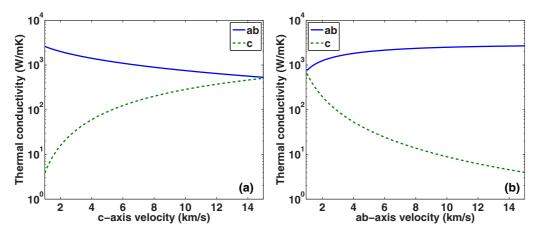
FIG. 1. (Color online) Thermal conductivity of graphite along the ab axis and the c axis as (a) the c-axis velocity is varied and the ab-axis velocity is fixed at 15 km/s, and (b) the ab-axis velocity is varied and the c-axis velocity is fixed at 1 km/s. Decreasing the c-axis velocity increases the ab-axis thermal conductivity, while decreasing the ab-axis velocity increases the c axis thermal conductivity.
