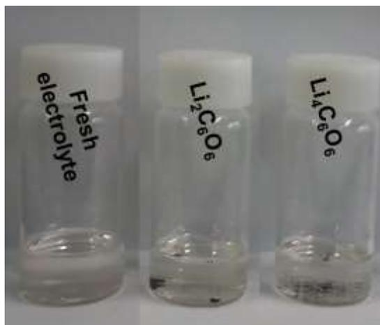
**Figure S7.** Photo image of Fresh electrolyte and the electrolyte storing Li<sub>2</sub>C<sub>6</sub>O<sub>6</sub> and Li<sub>4</sub>C<sub>6</sub>O<sub>6</sub> for 48 hours (from left to right).
