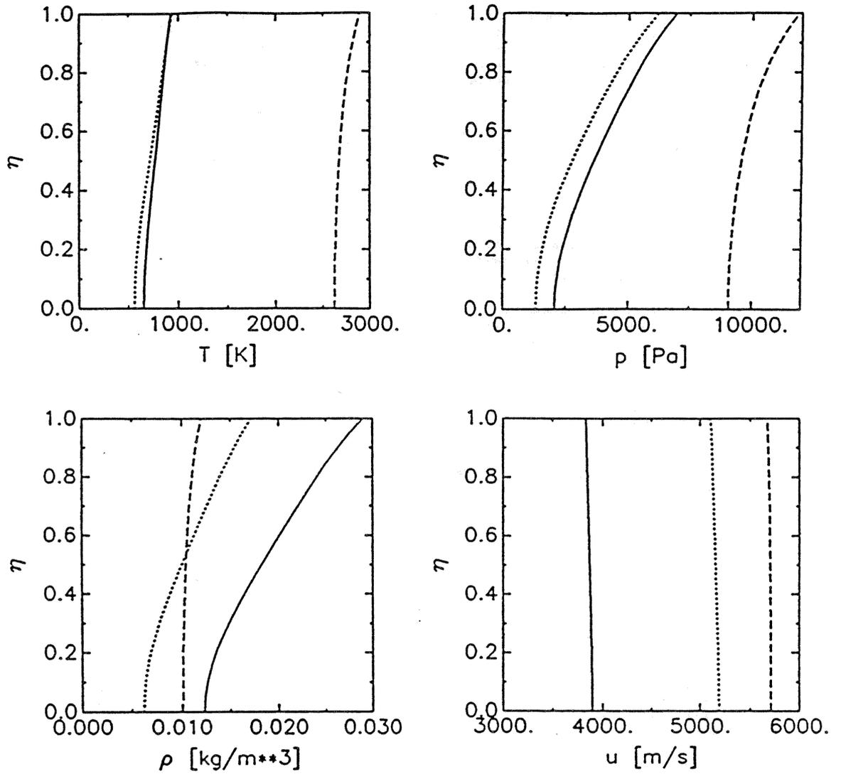
Fig. 11: Ideal gas flow, state variables versus non-dimensional radius at the nozzle exit (solid lines), comparison with partial equilibrium flow,  $\lambda_{crit} = 0.1m$ , (dashed lines) and frozen flow (dotted lines)
