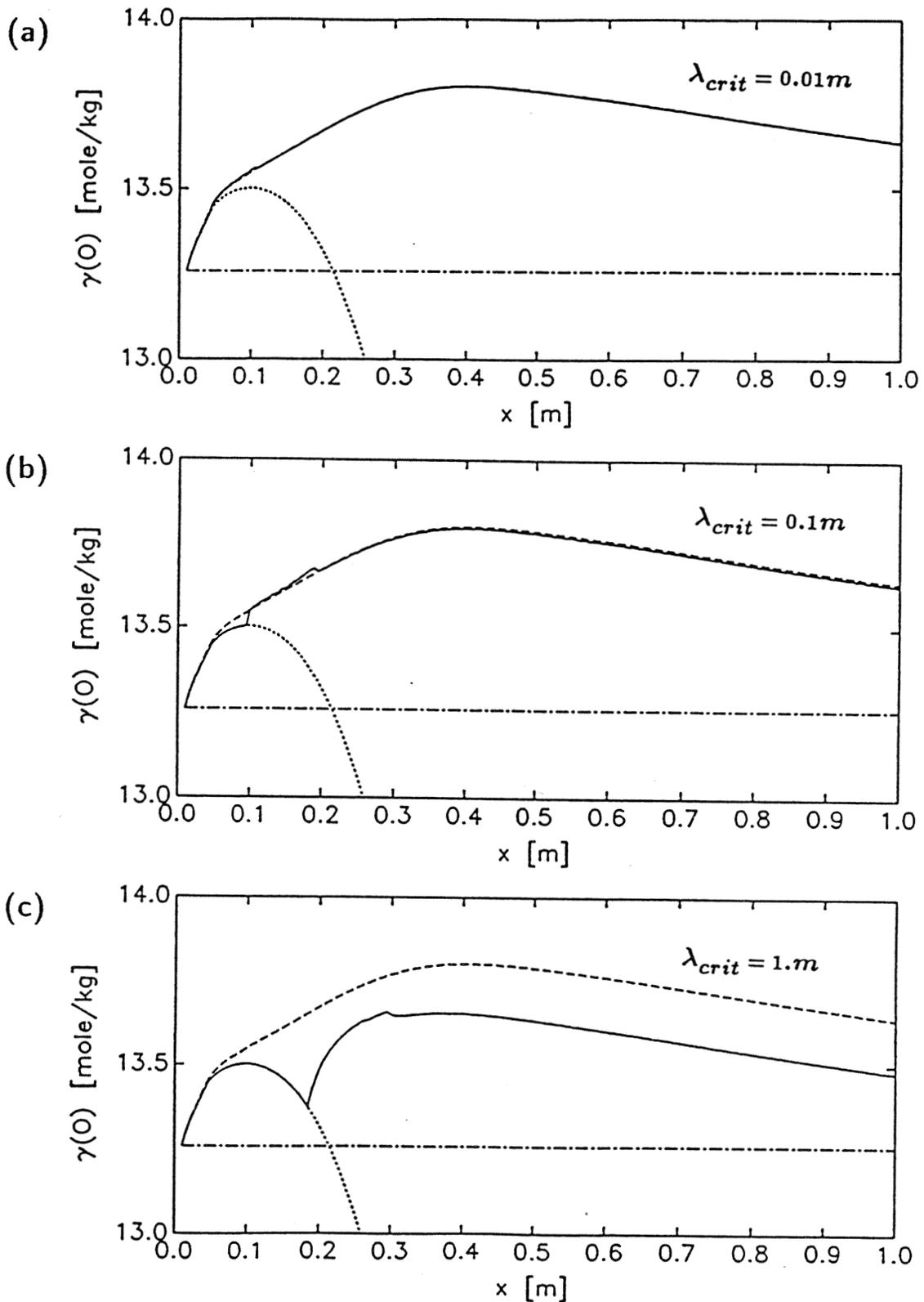
Fig. 7: Concentration  $\gamma_O$  of monatomic oxygen along nozzle axis, comparison of partial equilibrium flow (solid line), equilibrium flow (dotted line), nonequilibrium flow (dashed line) and frozen flow (chain-dotted line): (a)  $\lambda_{crit} = 0.01m$ , (b)  $\lambda_{crit} = 0.1m$ , (c)  $\lambda_{crit} = 1.m$
