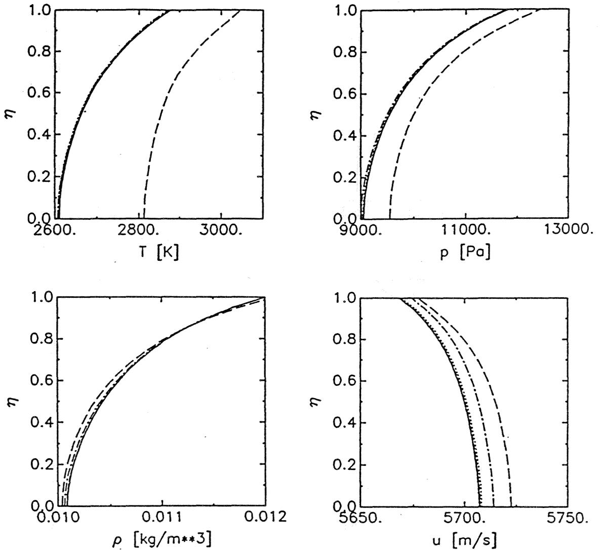
Fig. 8: State variables versus non-dimensional radius  $\eta$  at the nozzle exit: comparison of nonequilibrium flow (solid lines) and partial equilibrium flows with  $\lambda_{crit} = 0.01m$  (short-dashed lines),  $\lambda_{crit} = 0.1m$  (dotted lines),  $\lambda_{crit} = 1m$  (chain-dotted lines),  $\lambda_{crit} = 10m$  (long-dashed lines)
