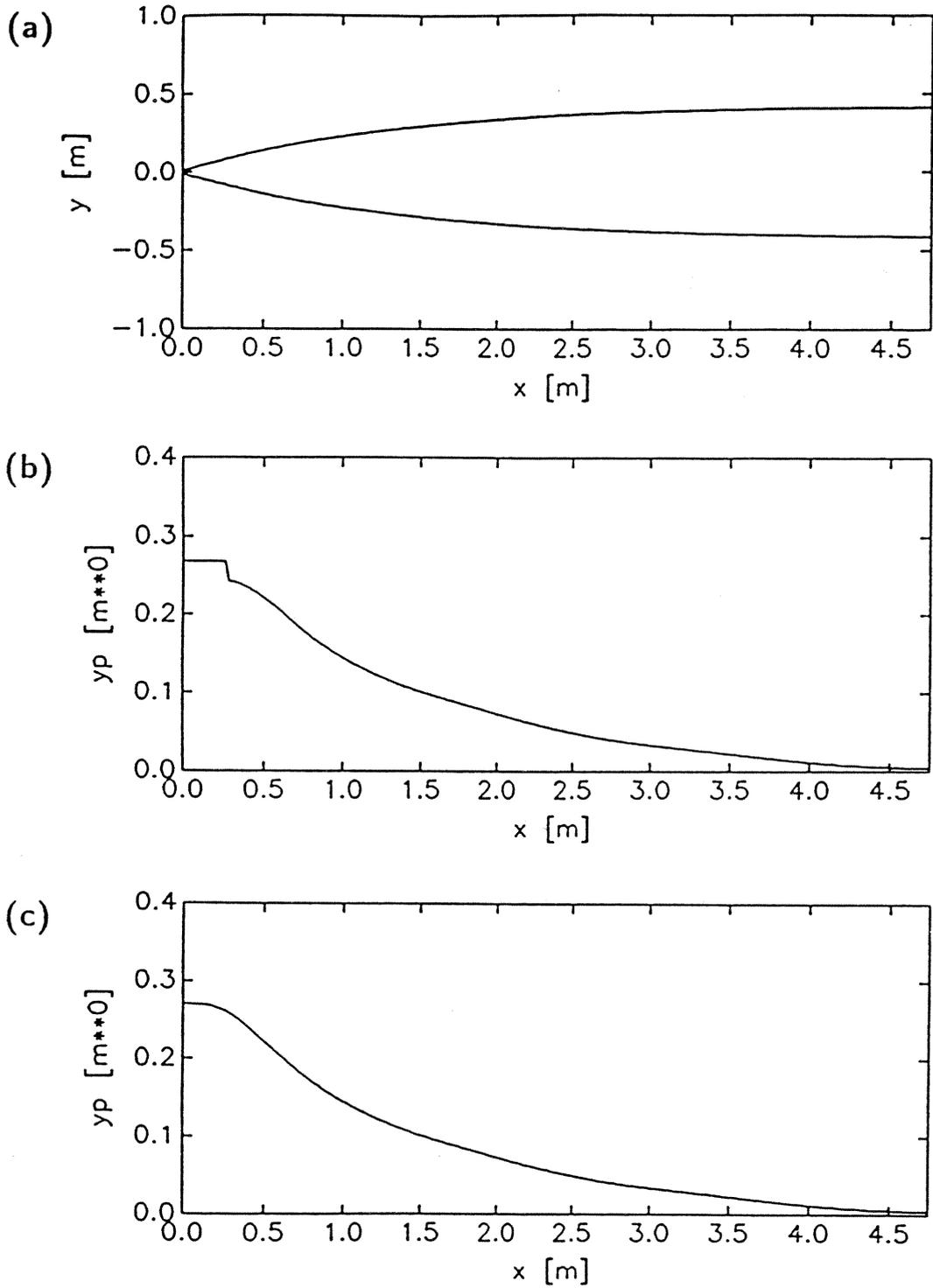
Fig. 19: Nozzle of the HEG shock tunnel:
