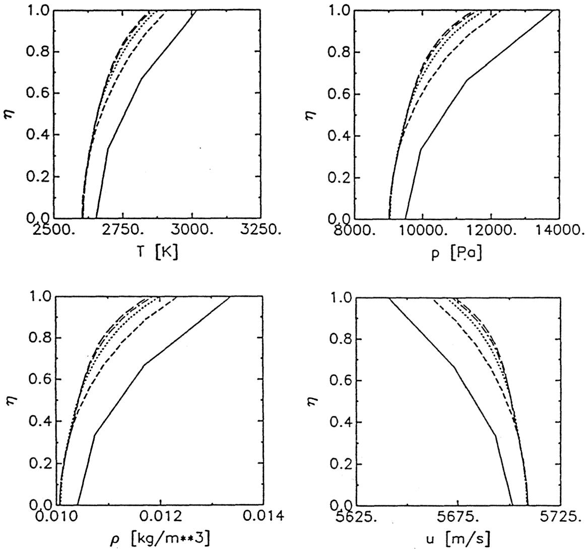
Fig. 18: Different number  $n_{max}$  of lines (standard case): state variables versus non-dimensional radius  $\eta$  at the nozzle exit ( $n_{max} = 4$ : solid lines,  $n_{max} = 10$ : short-dashed lines,  $n_{max} = 20$ : dotted lines,  $n_{max} = 30$ : chain-dotted lines,  $n_{max} = 40$ : long-dashed lines)
