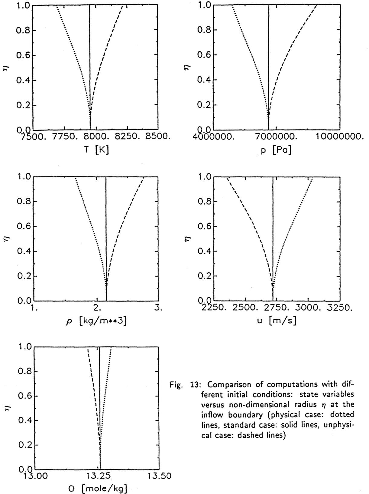
Fig. 13: Comparison of computations with different initial conditions: state variables versus non-dimensional radius  $\eta$  at the inflow boundary (physical case: dotted lines, standard case: solid lines, unphysical case: dashed lines)
