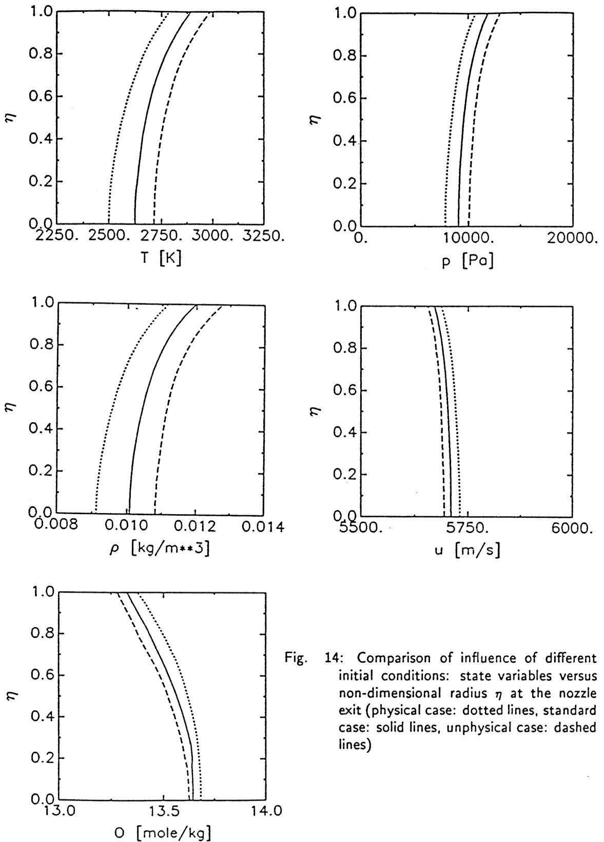
Fig. 14: Comparison of influence of different initial conditions: state variables versus non-dimensional radius  $\eta$  at the nozzle exit (physical case: dotted lines, standard case: solid lines, unphysical case: dashed lines)
