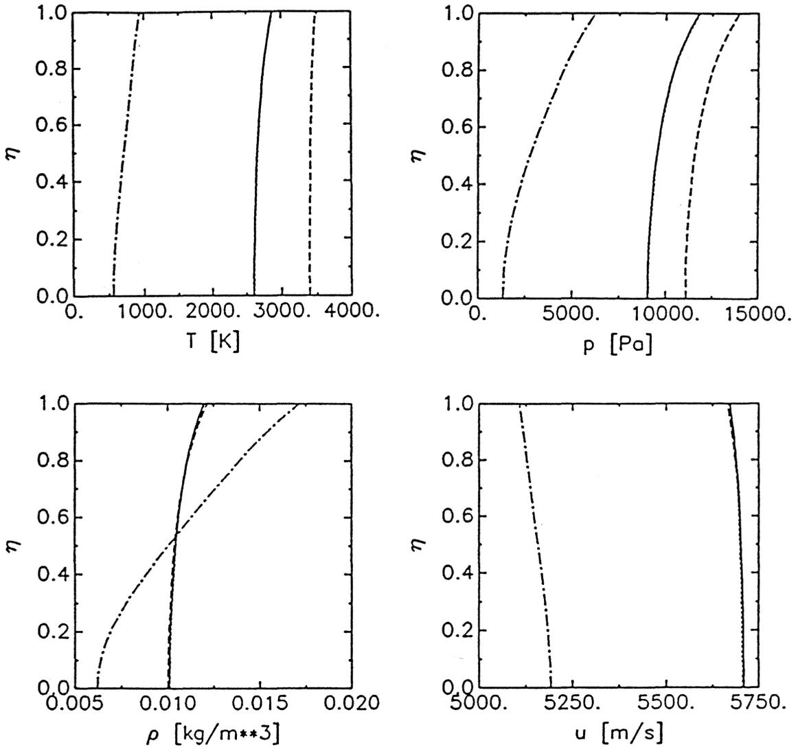
Fig. 4: Partial equilibrium flow,  $\lambda_{crit} = 0.1m$  (standard case): state variables versus non-dimensional radius  $\eta$  at the nozzle exit (solid lines), comparison with nonequilibrium flow (dotted lines), equilibrium flow (dashed lines) and frozen flow (chain-dotted lines) [the partial equilibrium flow solution cannot always be distinguished from the nonequilibrium solution, further, the frozen flow solution is not always plotted]
