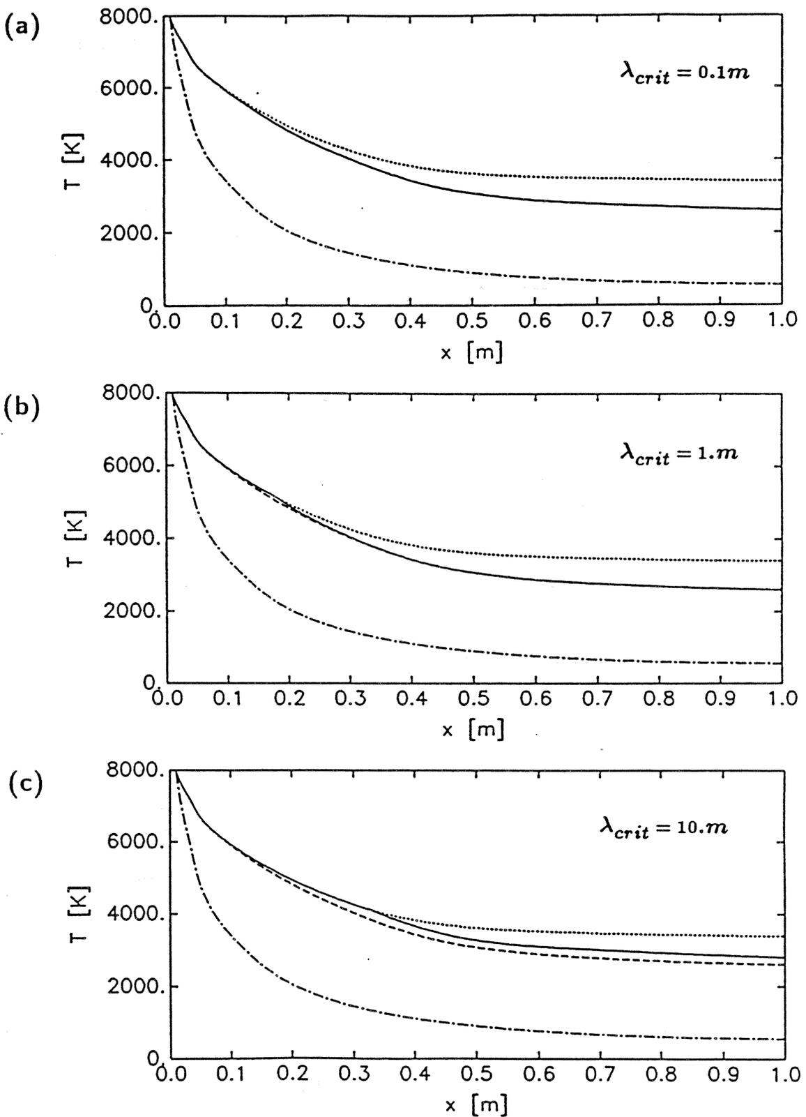
Fig. 6: Temperature along nozzle axis, comparison of partial equilibrium flow (solid line), equilibrium flow (dotted line), nonequilibrium flow (dashed line) and frozen flow (chain-dotted line): (a)  $\lambda_{crit} = 0.1m$ , (b)  $\lambda_{crit} = 1.m$ , (c)  $\lambda_{crit} = 10.m$
