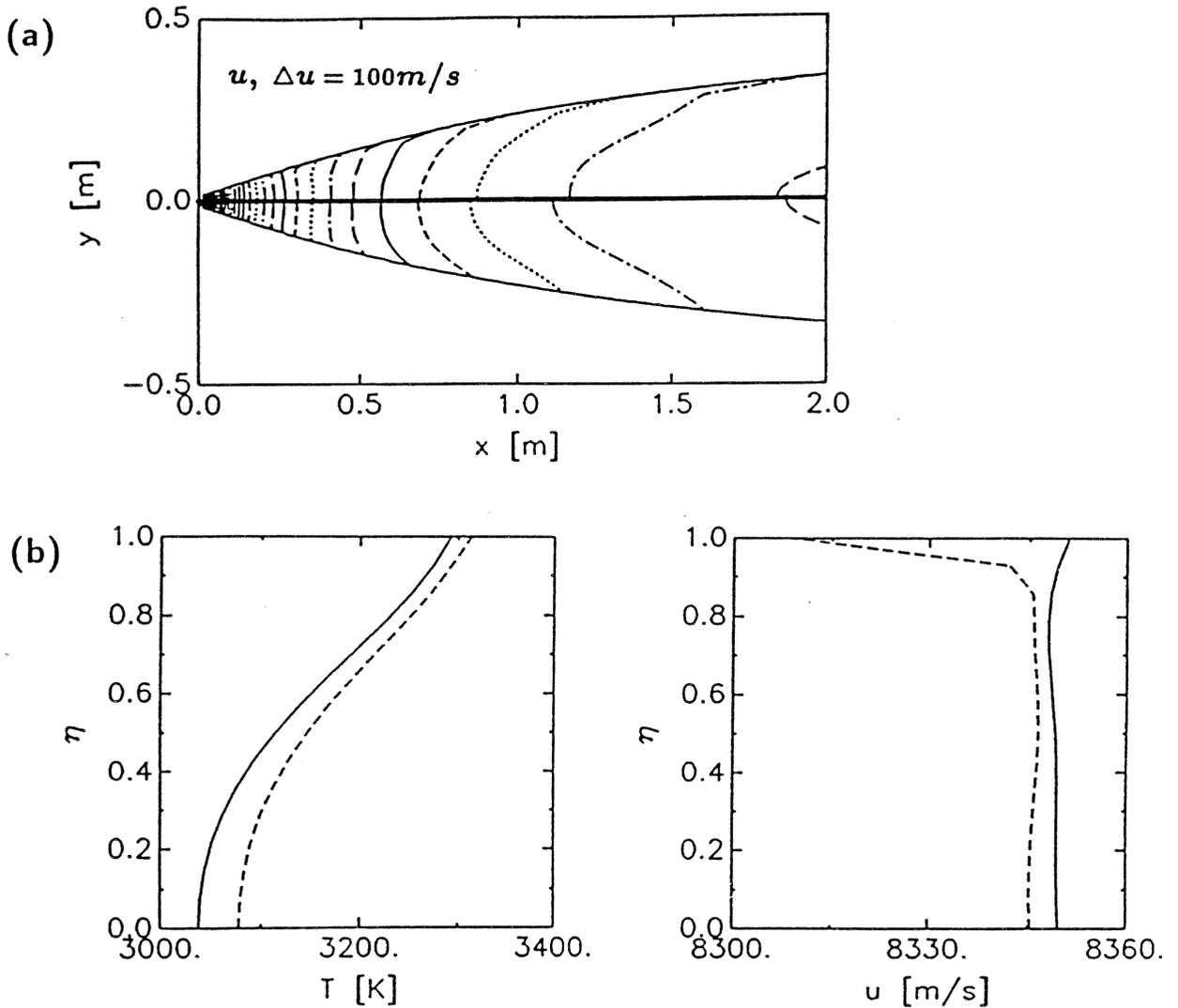
Fig. 20: Comparison of results obtained by a computation of a flow through two different versions of the nozzle of the HEG shock tunnel:
