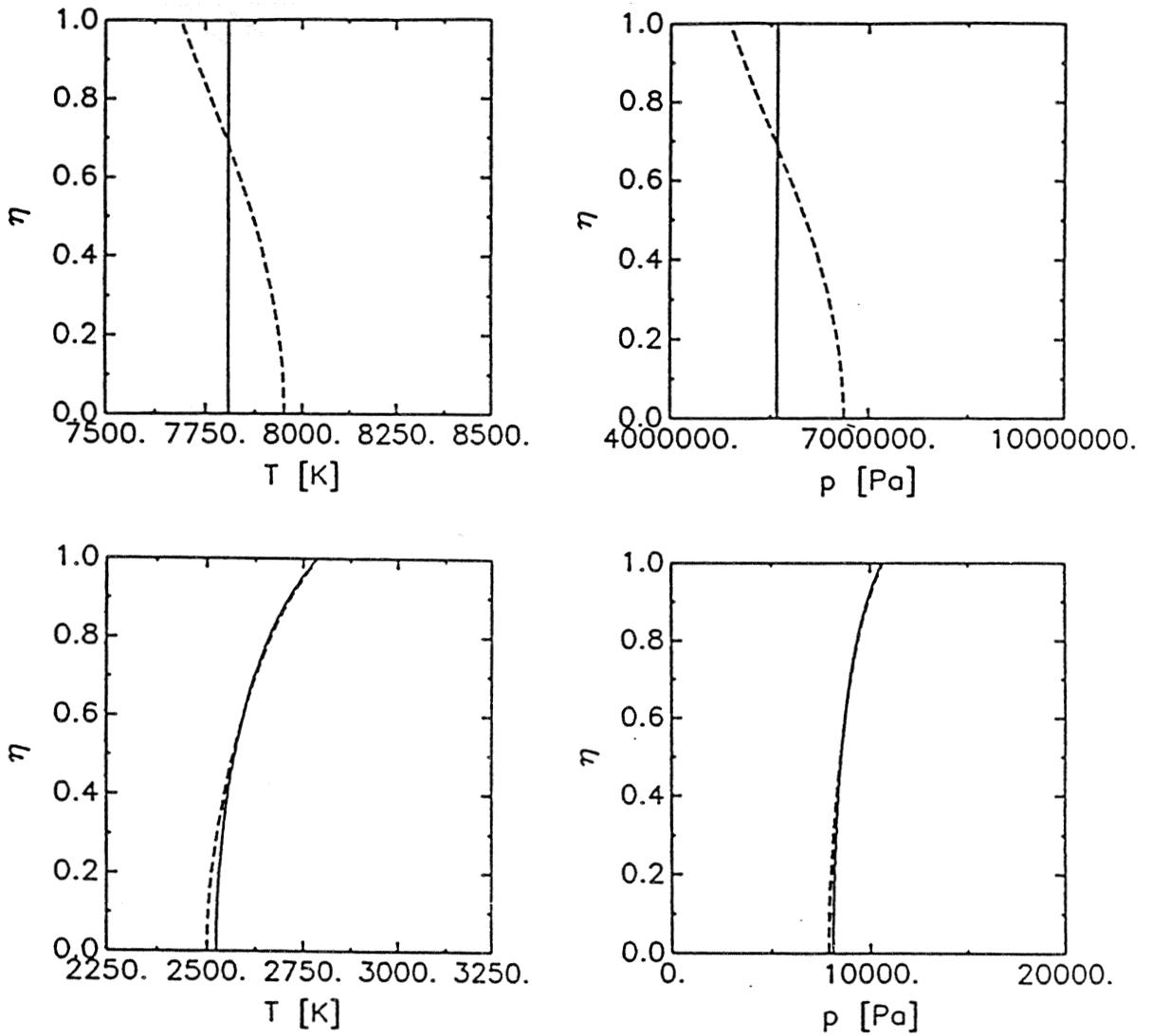
Fig. 17: Different initial conditions but same energy flux at inflow boundary: temperature and pressure versus non-dimensional radius  $\eta$ :
