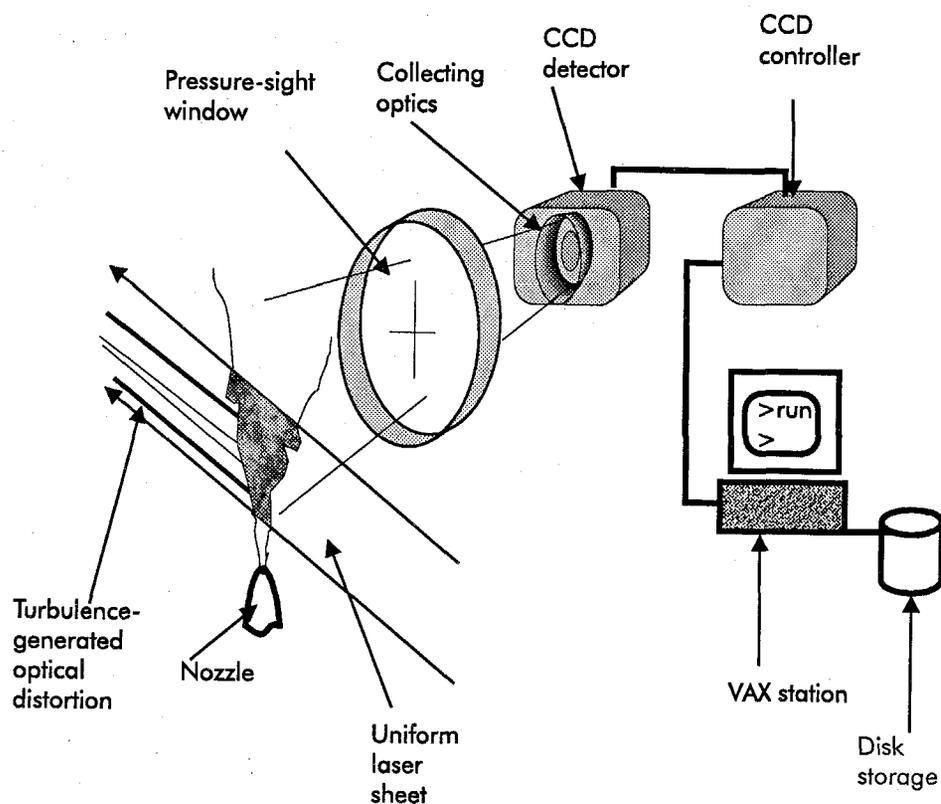
FIG. 1 Experimental set-up.
