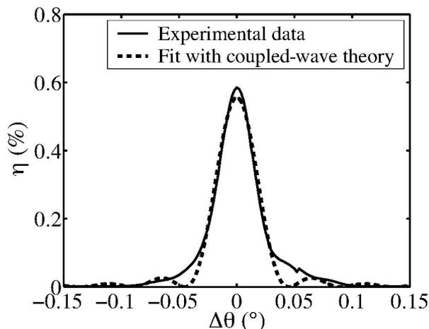
Fig. 2. Diffraction efficiency  $\eta$  versus readout angle  $\Delta\theta = (\theta - \theta_B)$  for a Foturan sample at the readout wavelength  $\lambda = 633$  nm. The dashed curve is a fit of the coupled-wave theory<sup>8</sup> to the experimental data (fit parameters  $d = 0.63$  mm and the grating amplitude).
