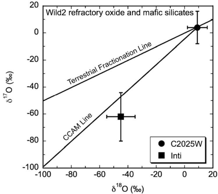
Fig. S5. Oxygen isotope compositions of refractory inclusion “Inti” and Mg-rich vesicular glass, determined by NanoSIMS. Inti is enriched in  $^{16}\text{O}$ , similar to refractory inclusions in chondritic meteorites, while the vesicular glass has a composition similar to mafic silicates in carbonaceous chondrites. Uncertainties are  $2\sigma$ .
