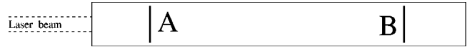
FIG. 1. Identical defects A and B create fluctuating stress in different parts of the test mass. The stress created by defect A will influence the phase shift of the laser beam readout more than the stress created by defect B , although both A and B make identical contributions to the Q 's of the test-mass elastic modes.
