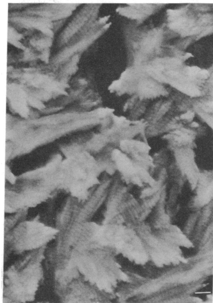
FIG. 5. High-magnification view of a 24-hr NaOCl-treated specimen, showing discontinuous clusters of banded material, which in part is covered with an apparently organic coating. Note also the sharp ends of some of the clusters. The specimen was imaged uncoated in a field emission SEM. (Bar = 100 nm.)
