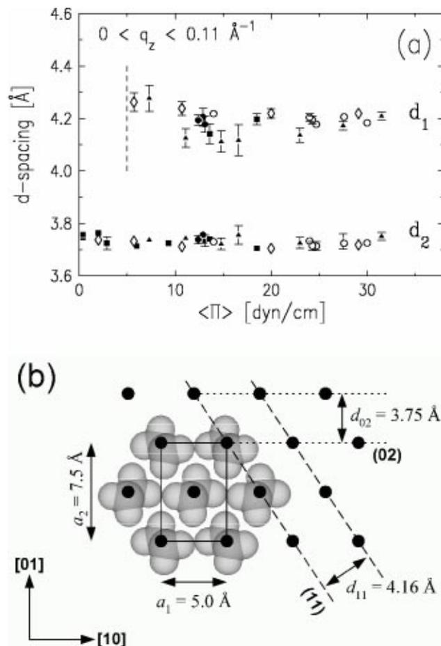
FIG. 14. (a) The  $d$  spacing  $d_1=2\pi/q_1$  and  $d_2=2\pi/q_2$  extracted from the GID measurements on C16-O-PBLG monolayers: PD325 films at 22.5 °C (filled symbols) and MD76 films at 22.5 °C (open circles) and at 30.9 °C (open diamonds). (b) End-on view of the HB packing arrangement of alkyl chains and the rectangular HB unit cell.
