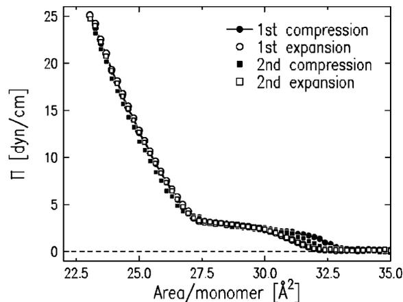
FIG. 3. Compression/expansion isotherms taken on a C16–O–PBLG film (PD325) at  $22^\circ\text{C}$  (the same film for all scans). The film was compressed only up to  $\Pi=25 \text{ dyne/cm}$ , and went through two compression/expansion cycles.
