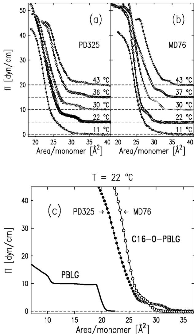
FIG. 2.  $\Pi$ - $A$  isotherms from C16–O–PBLG monolayers: (a) PD325 films and (b) MD76 films at various temperatures (shifted vertically for clarity); (c) room-temperature comparison between PD325 and MD76 films of C16–PBLG and bare PBLG.
