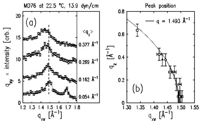
FIG. 15. (a)  $q_{xy}$  scans at various height  $\langle q_z \rangle$  above the surface (vertically shifted for clarity) measured on a MD76 film at 22.5 °C and  $\Pi=13.9$  dyne/cm. (b) Peak positions in reciprocal space: MD76 films at 13.9 dyne/cm (open circles) and at 24.0 dyne/cm (open squares), and a PD325 film at 31.3 dyne/cm (filled triangles), all at 22.5 °C.
