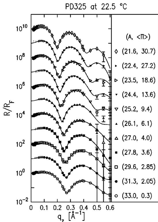
FIG. 5. Specular reflectivity normalized to the Fresnel reflectivity, measured from C16–O–PBLG films (PD325) at 22.5 °C and at various area/monomer  $A$  or surface pressure  $\Pi$  (shifted vertically for clarity). The solid lines are the best-fit  $R/R_F$  curves based on a two-box model for the average electron density profiles  $\langle \rho(z) \rangle$ .
