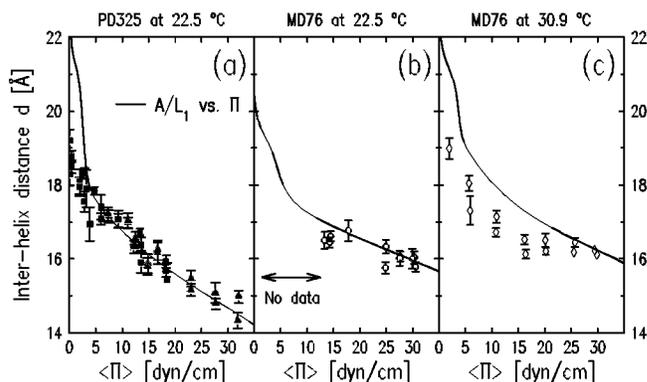
FIG. 12. Interhelix  $d$  spacing vs  $\Pi$  for C16–O–PBLG monolayers: (a) PD325 films at 22.5 °C, (b) MD76 films at 22.5 °C, and (c) MD76 films at 30.9 °C. Each solid line is given by dividing the area from isotherm by the helical pitch  $L_1 = 1.5 \text{ \AA/monomer}$  along the helical axis.
