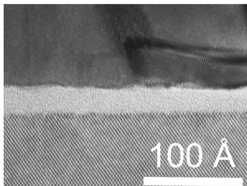
Fig. 3. XTEM photomicrograph of sample II, 1000 Å Ni/20 Å Ga<sub>2</sub>O<sub>3-x</sub>/p-GaAs.
