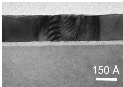
Fig. 2. XTEM photomicrograph of sample I. The bottom layer is the intrinsic GaAs buffer layer. The topmost layer is the 175-Å-thick Au cap. Between these layers, the 20-Å-thick Ga<sub>2</sub>O<sub>3-x</sub> layer is seen to be distinct and fairly smooth.
