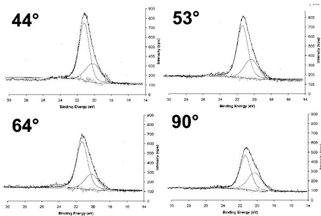
FIG. 7. Deconvolution of the Ga  $3d$  transition in sample II measured by an angle-resolved scan using a Mg  $K\alpha$  source; see Table III. The rightmost (lower-energy) curves are presumed to originate from Ga bonded to As, while the leftmost (higher-energy) curves are presumed to originate from Ga bonded to O.
