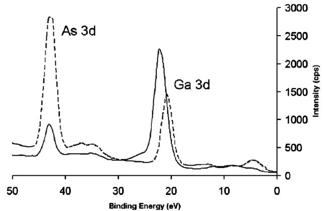
FIG. 6. XPS scans of sample I before and after e-beam evaporation of  $\text{Ga}_2\text{O}_3$ . The dashed line represents the GaAs surface prior to evaporation, the solid line the sample surface after oxide film deposition.
