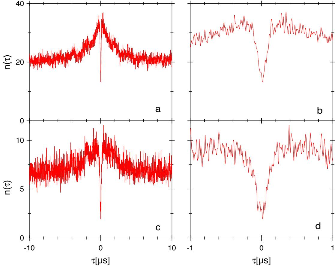
FIG. C: Coincidence counts  $n(\tau)$  versus time offset  $\tau$  obtained from the recorded photoelectric events at detectors  $D_{1,2}$ . These data were used to obtain  $g^{(2)}(\tau)$  in Fig. 4 of our paper [1].
