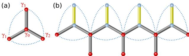
FIG. 2. (Color online) (a) Minimal implementation required for braiding with the shortcut protocol. The additional couplings needed for the shortcut protocol are shown in blue. (b) Wire network with many Majoranas allowing for pairwise exchanges of neighboring Majoranas including the shortcut protocol. Implementing the shortcut merely requires the addition of local couplings within the network.
