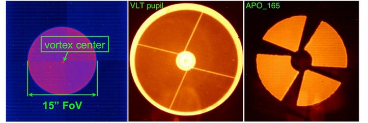
**Fig. 2.** Left: view from inside CONICA, showing the 9 mm clear aperture corresponding to a  $15''$  field of view (diameter), fully contained within the  $27''$  field of view of the L27 objective. Middle: full oversized stop of CONICA, showing the VLT pupil (including the central obscuration and struts). Right: APO165 pupil mask (diameter =  $0.87 \times D_{pup}$ ) available inside CONICA, aligned to cover the diffraction and thermal background from the central obscuration and struts.
