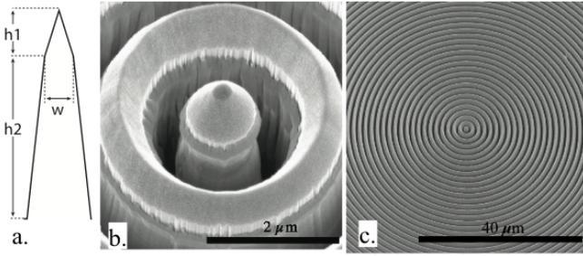
**Fig. 1.** Scanning electron microscope (SEM) images of the NACO AGPM. a. Structure profile schematic, with  $h_2 = 5 \pm 0.1 \mu\text{m}$ ,  $h_1 = 1 \pm 0.1 \mu\text{m}$ , and  $w = 0.65 \pm 0.03 \mu\text{m}$  (the grating pitch is  $1.42 \mu\text{m}$ ). b. Zoom on the center of the diamond AGPM. c. Overview of the structure showing the uniformity and original cleanliness of this particular device.
