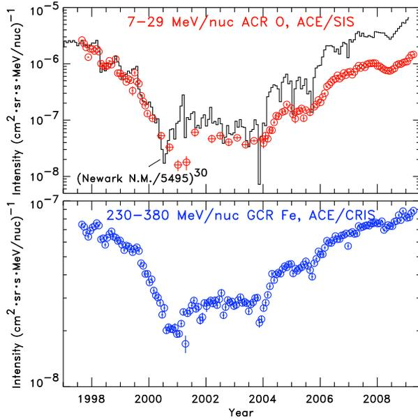
Fig. 1. Bartels rotation averages of quiet-time 7-29 MeV/nucleon oxygen (mostly ACRs) from ACE/SIS (*top panel*) and 230-380 MeV/nucleon iron (GCRs) from ACE/CRIS (*bottom panel*). Also shown in the *top panel* is the Newark neutron monitor rate, scaled as indicated.
