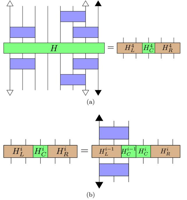
FIG. 17. Fig. 17(a) shows an example of an effective Hamiltonian centered at site 4 for the GDMRG algorithm. The example is for  $N = 8$  sites and a block size of  $B = 3$ . Here the center is only one site, but could be more to improve convergence just like in the standard DMRG algorithm. Fig. 17(b) shows, for a sweep to the right, how to obtain the new left block from the previous effective Hamiltonian.
