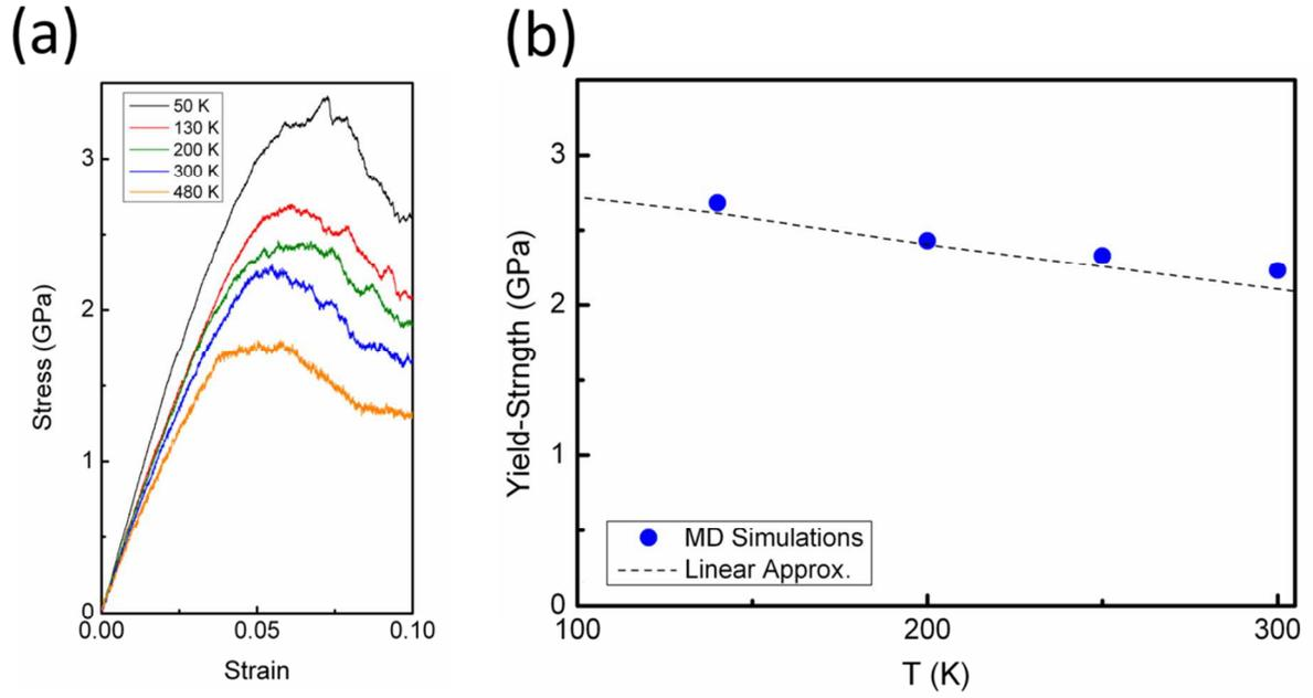
**Fig. S1** | (a) Engineering stress-strain curves for the  $\text{Cu}_{60}\text{Zr}_{40}$  metallic glass under uniaxial compression test at different temperatures from 50 K to 480 K. (b) Variation of yield strength,  $\sigma_y$ , with temperature at the temperature range of our experiments (130 K-300 K) obtained from molecular dynamics (scattered dots) and the suggested linear approximation to explain the experimental results (dashed-line).
