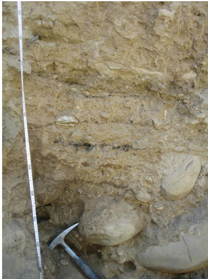
Figure S34: Close-up of sample location near present-day river bed. Dark layers near the center of the photograph contains charcoal pieces, which have been sampled.
