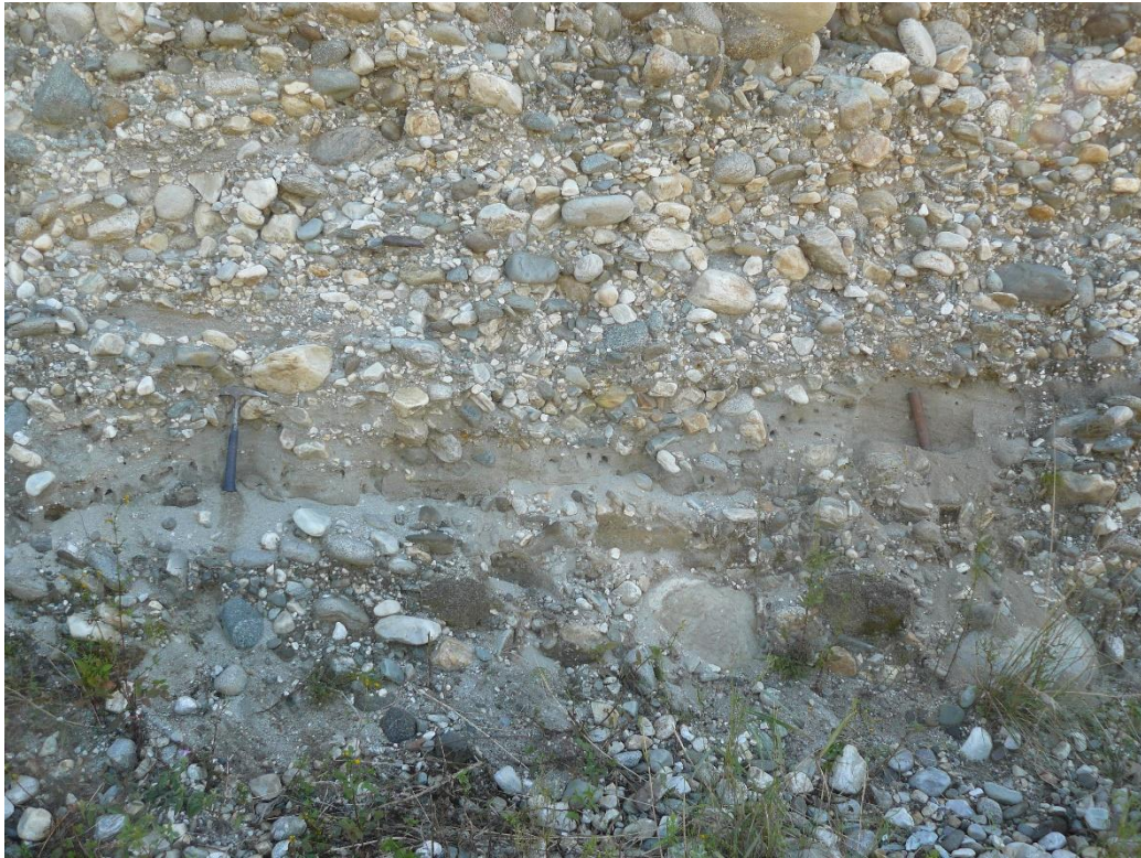
Figure S26: Coarse-sand lens (25 cm thick) where sample was taken from. See hammer on the left for scale and tube on the right for sampling location.
