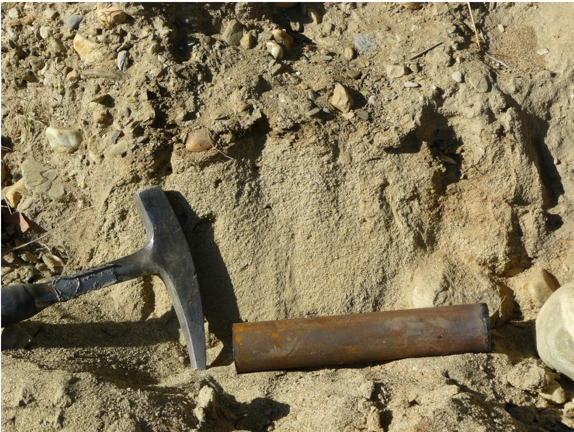
Figure S19: Close-up of ~20 cm thick medium-sand lens where sample was taken from.
