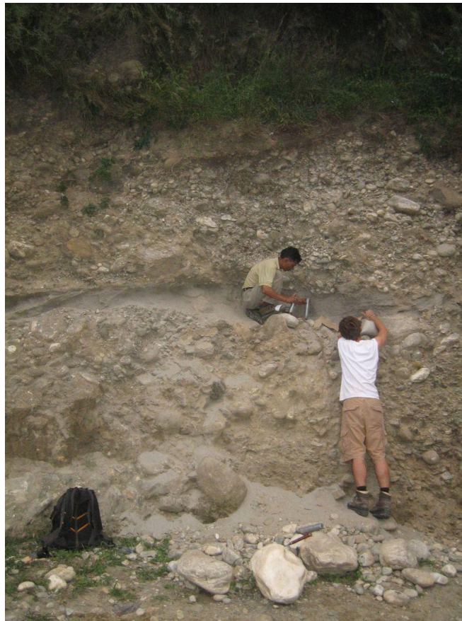
Figure S17: Sand sample for paleo-erosion rates was sampled from sand lens that was imbedded in light-colored Yamuna deposits. We attempted to collect a tube sample (see photo) for dating the deposits, but aborted the plan due to unsafe conditions during hammering the tube into the deposits.
