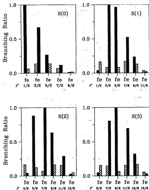
FIG. 8. Calculated rotational branching ratios resulting from  $(2 + 1')$  REMPI of HBr via the  $S(n)$ ,  $n = 0 - 3$ , rotational branches of the  $F^1\Delta_2$  intermediate state. The kinetic energy of the photoelectron is 50 meV. Other notations are the same as in Fig. 1.
