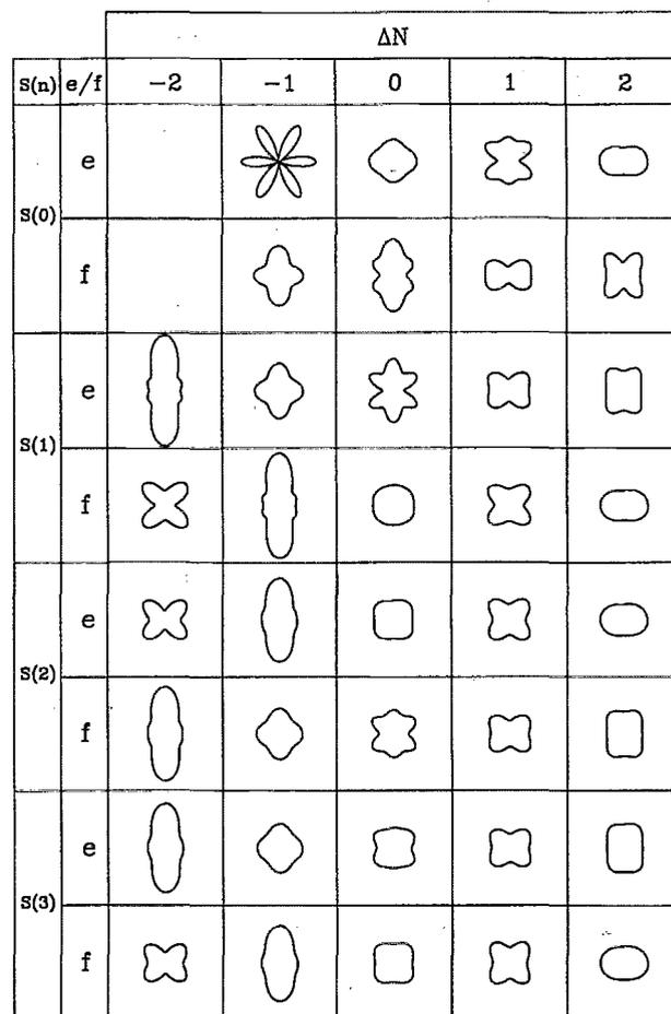
FIG. 9. Calculated photoelectron angular distributions corresponding to the rotational ion distributions of Fig. 8. Asymmetry parameters up to  $\beta_6$  are evaluated.  $\Delta N = N^+ - N' = J^+ + \frac{1}{2} - J'$  with  $N' = J = n + 2$  for the  $S(n)$ ,  $n = 0 - 3$ , branches. The polarization direction is vertical ( $\theta = 0$ ).
