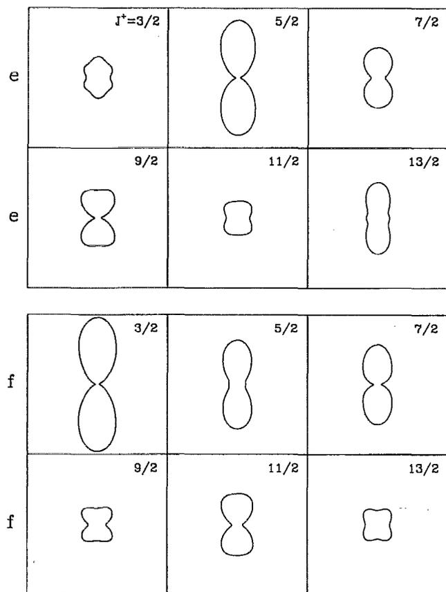
FIG. 6. Calculated photoelectron angular distributions for the rotational levels of Fig. 1. The polarization direction is vertical ( $\theta = 0$ ).
