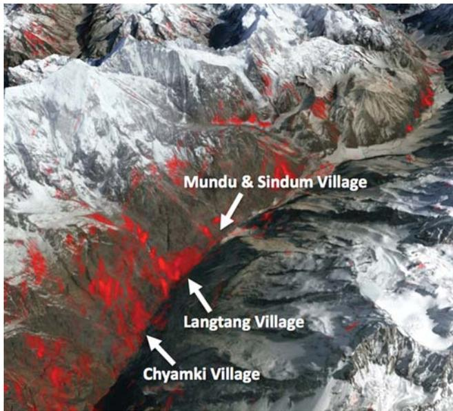
▲ **Figure 6.** Perspective view of Langtang valley with the ALOS-2 DPM (red pixels as shown in Fig. 5) draped on Google Earth. Chyamki, Langtang, Mundu, and Sindum villages were reported to be damaged by induced landslides.
