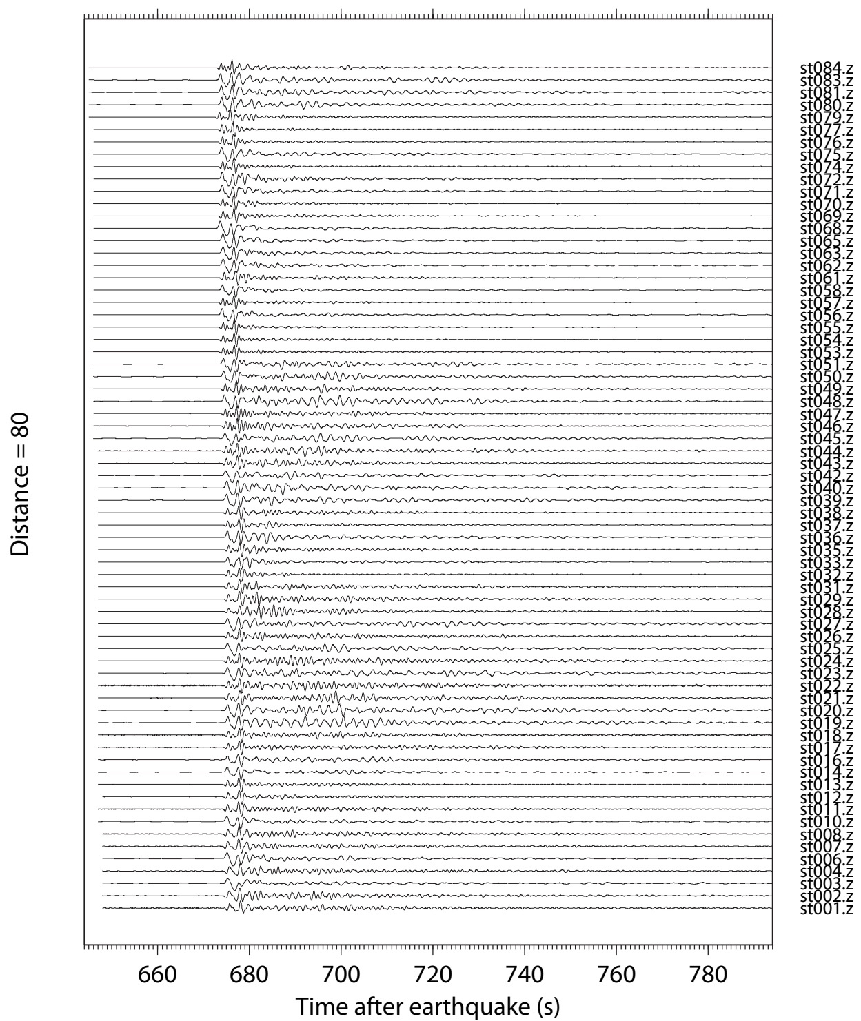
Figure 4i. Vertical-component record section for teleseismic event which occurred on April 8, 1999 on the Eastern Russia-China border (Event_1999.04.08.13.10.34.00).
