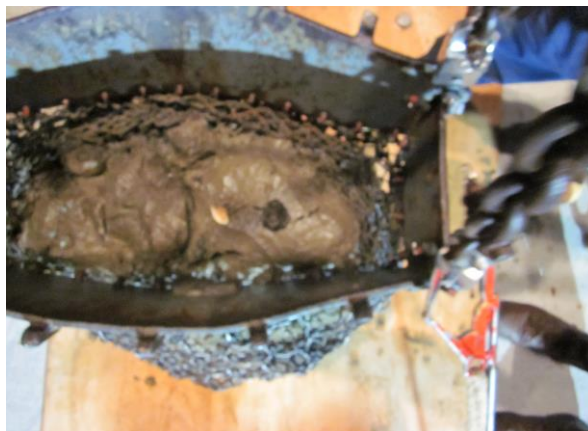
Figure 7. Dredge bag containing fine mud and rock samples collected from around the OBS04 location of 33^{\circ} 19.12' \text{ N} , -119^{\circ} 10.97' \text{ W} , and depth of approximately 1200 m.
