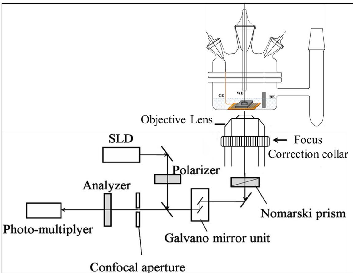
**Figure S2** Schematic diagram of LCM-DIM system combined with electrochemical cell. To achieve atomic-height resolution in solution, a specially designed objective lens with a compensator (focus correction collar) was used to adjust the focus point caused by changes in the refraction index by the solution and the glass plate.
