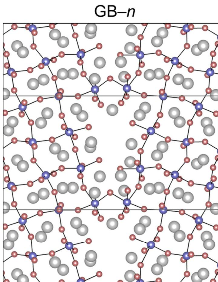
**Fig. S3.** Structure of grain boundary with surplus cations. This can be thought as adding more Rb into  $GB-N$  (Fig. 3).
