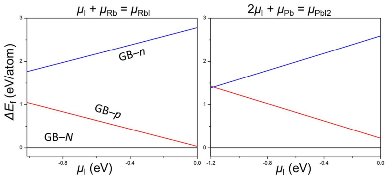
**Fig. S5.** Energies of various grain boundaries, with respect to that of  $GB-N$ , as a function of  $I$  chemical potential (with respect to that of  $I_2$  molecule) along phase boundaries.
