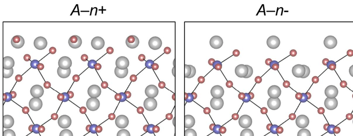
**Fig. S1.** Edges along  $A$  direction with surplus cations/deficient anions.  $A-n+$  can be thought as adding more Rb into  $A-N+$  (Fig. 2), and  $A-n-$  can be thought as removing I from  $A-N+$ , or adding more Rb into  $A-N-$  (Fig. 2).
