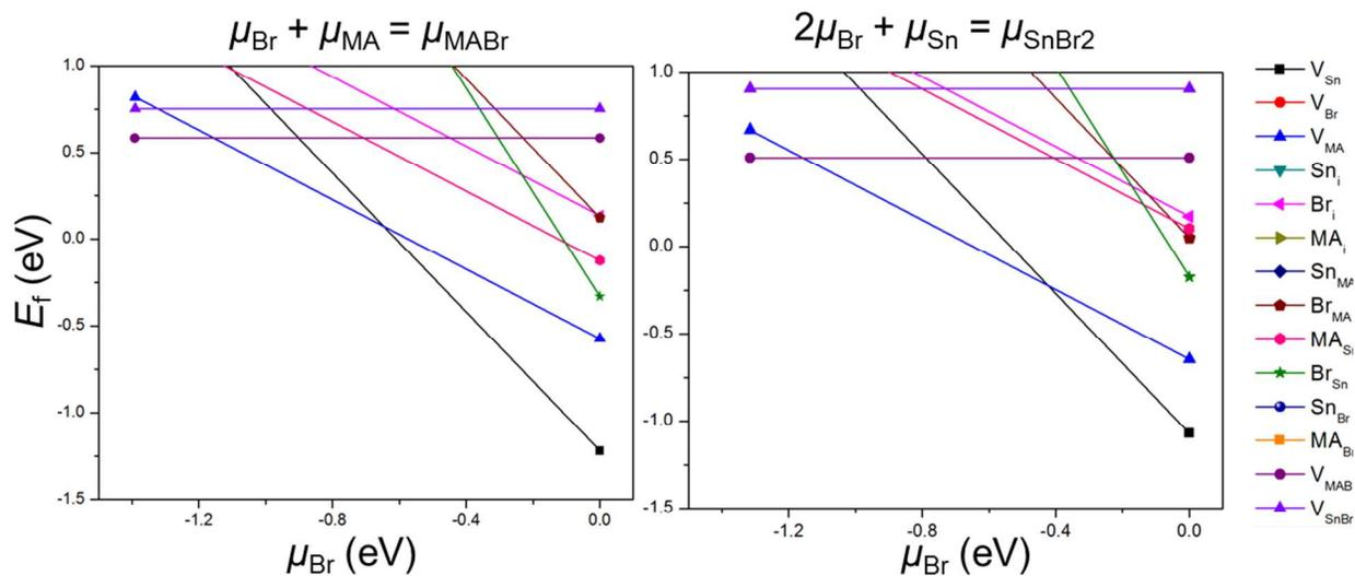
**Fig. S6.** Energies of various point defects in 2D  $\text{MA}_2\text{SnBr}_4$  ( $\text{MA} = \text{CH}_3\text{NH}_3$ ), as a function of Br chemical potential (with respect to that of  $\text{Br}_2$  molecule) along phase boundaries. These suggest that the formation of harmful defects can be suppressed by decreasing the chemical potential of Br, in consistence with  $\text{Rb}_2\text{PbI}_4$ .
