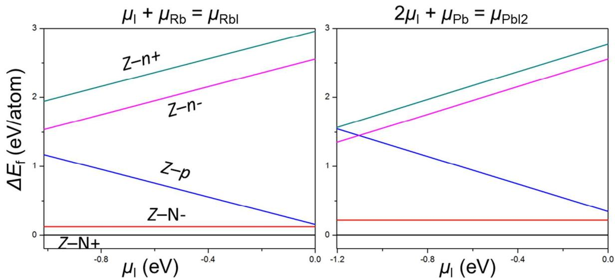
**Fig. S4.** Energies of various edges along  $Z$  direction, with respect to that of  $Z-N+$ , as a function of  $I$  chemical potential (with respect to that of  $I_2$  molecule) along phase boundaries.
