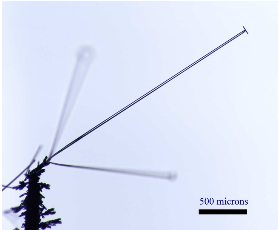
Figure 1: This photograph shows a typical c -axis ice needle crystal growing at -15 C. The supporting wire substrate is seen in the lower left of the photo, covered with a large number of frost crystals. Several thin, c -axis ice needles grew out from the wire tip, and one was brought into focus with the entire needle in the image plane. After 95 seconds of growth at a water-vapor supersaturation of \sigma_{center} \approx 11 percent (in this particular example) a thin ice plate can be seen growing on the tip of the ice needle, here seen in side view. The ice plate diameter, ice needle diameter below the plate, and the overall needle length can be extracted from a set of similar calibrated images.
