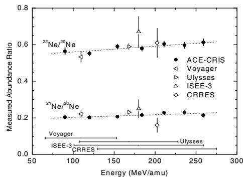
**Figure 2.** Our measurements of the isotope ratios  $^{22}\text{Ne}/^{20}\text{Ne}$  and  $^{21}\text{Ne}/^{20}\text{Ne}$  at the top of the CRIS instrument are plotted as a function of energy. The dotted lines are least squares fits to our data. Abundances measured by other experiments (see text for references) are plotted as open symbols. The energy intervals for their measurements are shown as horizontal bars at the bottom of the figure.
