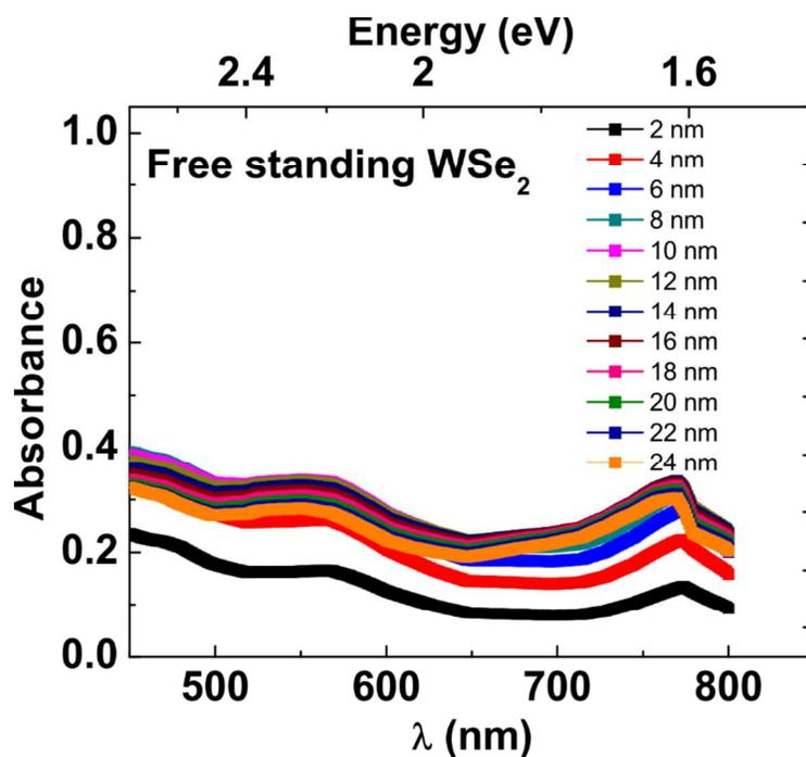
Figure S1: Calculated absorption in free standing WSe<sub>2</sub> with varying thickness. The total absorption increases with increasing thickness upto 12-14 nm and approaches ~40% following which it steadily drops down with further increase in the thickness.
