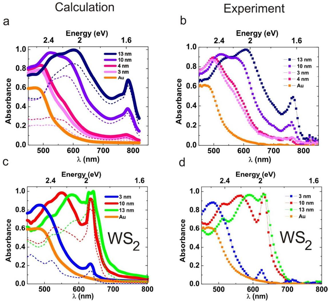
Figure S3: Calculated (left) and measured (right) absorption spectra of WSe<sub>2</sub> on Au (a-b) and WS<sub>2</sub> on Au(c-d).
