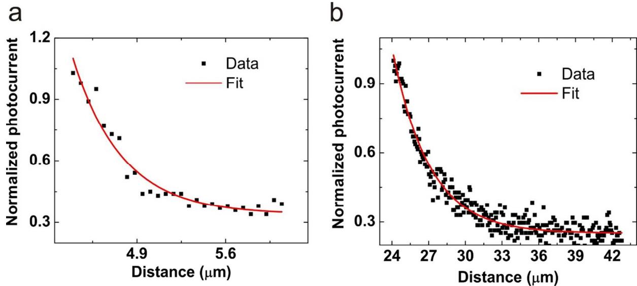
Figure S4. a. Photocurrent profile of device shown in Figure 3 e of the manuscript with a minority carrier diffusion length of  $\sim 1.35 \mu\text{m}$  b. Photocurrent profile of another representative device (19 nm  $\text{WSe}_2$  on Au) shown in Figure 4 e of the manuscript with a minority carrier diffusion length of  $\sim 3 \mu\text{m}$ .
