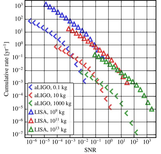
FIG. 1. Cumulative event rate for minimal (pure gravitational) interactions in a single Advanced LIGO detector and in a single LISA detector.  $\text{SNR} > 8$  correspond to very infrequent events, with rates below  $10^{-3} \text{ yr}^{-1}$  for aLIGO and  $10^{-1} \text{ yr}^{-1}$  for LISA.
