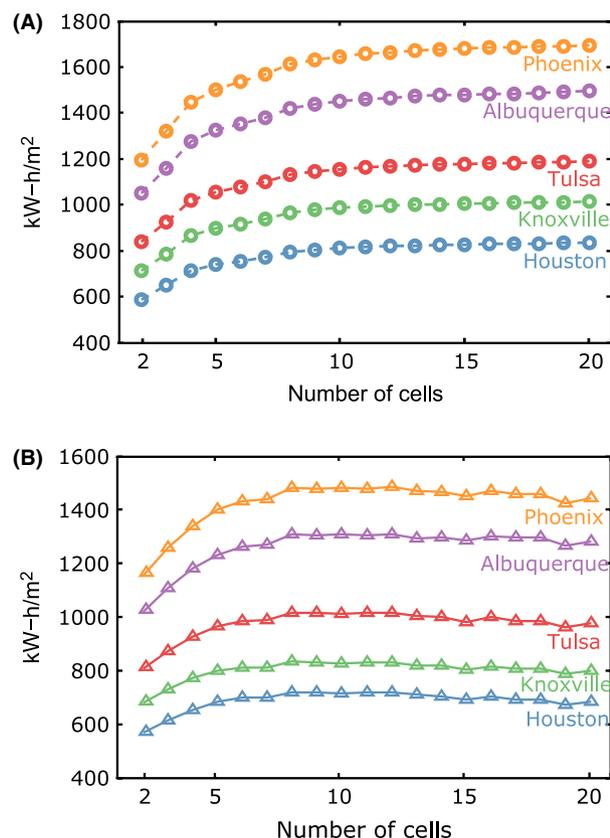
**Figure 5.** (A) Simulated annual energy production of ideal spectrum splitting ensembles with electrically independent subcells under 500 suns. Simulated spectra have intensity uniformly decreased by the average percent cloud coverage for each hour. (B) Simulated annual energy production of ideal spectrum splitting ensembles with series-connected subcells under cloud-adjusted spectra.
