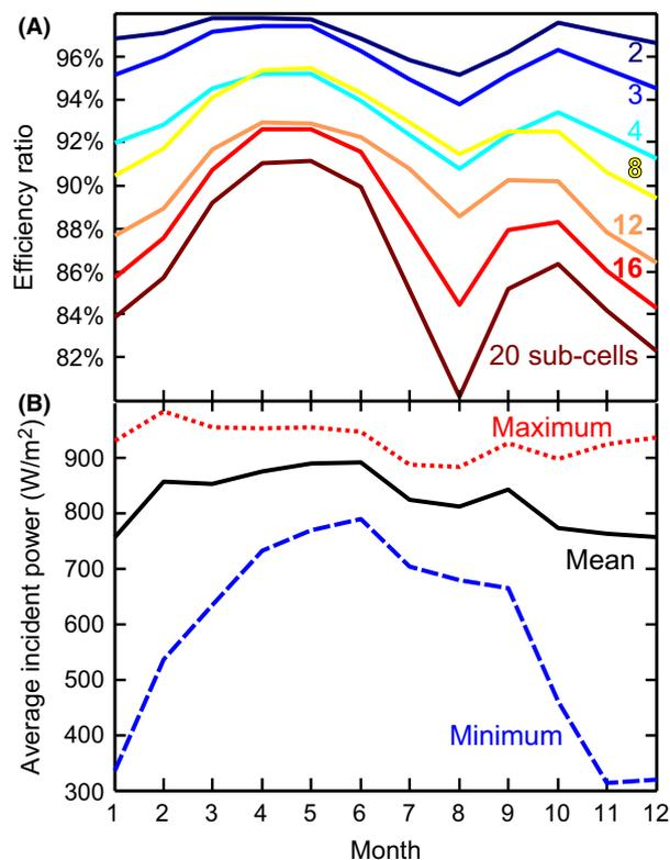
**Figure 3.** (A) Efficiency ratio of series-connected to electrically independent spectrum splitting ensembles averaged over all spectra in each month of the year in Phoenix, AZ. (B) Minimum, mean, and maximum irradiance level for each month of the year in Phoenix, AZ.
