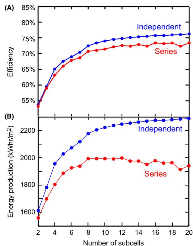
**Figure 1.** (A) Efficiency versus number of subcells for ideal spectrum splitting ensembles with electrically in series and independent subcells at 500 suns concentration under the AM1.5D spectrum. (B) Simulated annual energy production for Phoenix, AZ for electrically independent and in series spectrum splitting ensembles operating at 500 suns concentration. The energy production units are kWh/m<sup>2</sup> of aperture area.
