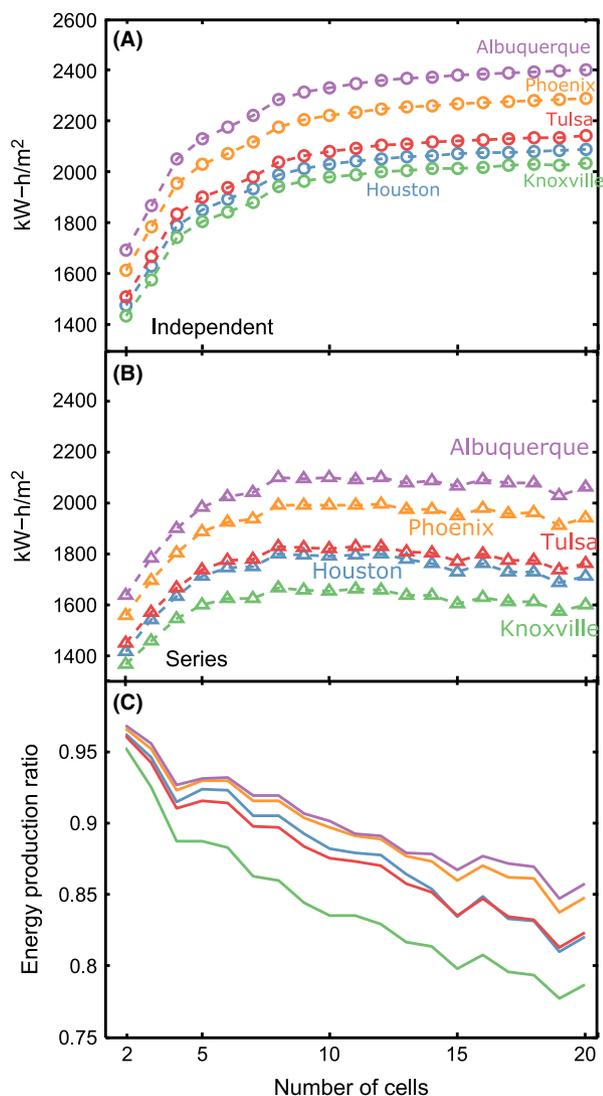
**Figure 4.** (A) Simulated annual energy production for ideal spectrum splitting ensembles with electrically independent subcells operating at 500 suns in Phoenix, AZ, Albuquerque, NM, Tulsa, OK, Knoxville, TN, and Houston, TX. All simulated spectra are for sunny days. (B) Simulated annual energy production for spectrum splitting ensembles with series-connected subcells. (C) Ratio of series-connected energy production to electrically independent energy production.
