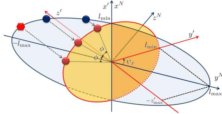
Fig. 2 Definition of  $\psi_x$  and the Relationship between the intermediate and the new frames
