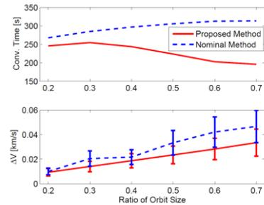
Fig. 5 Comparison of the performance: convergent time (upper figure) and fuel consumption (lower figure)
