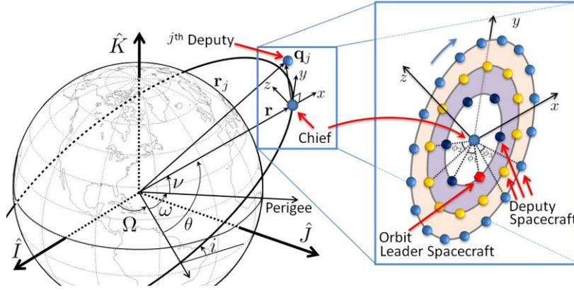
Fig. 1 Coordinate systems and spacecraft swarm in multiple concentric orbits
