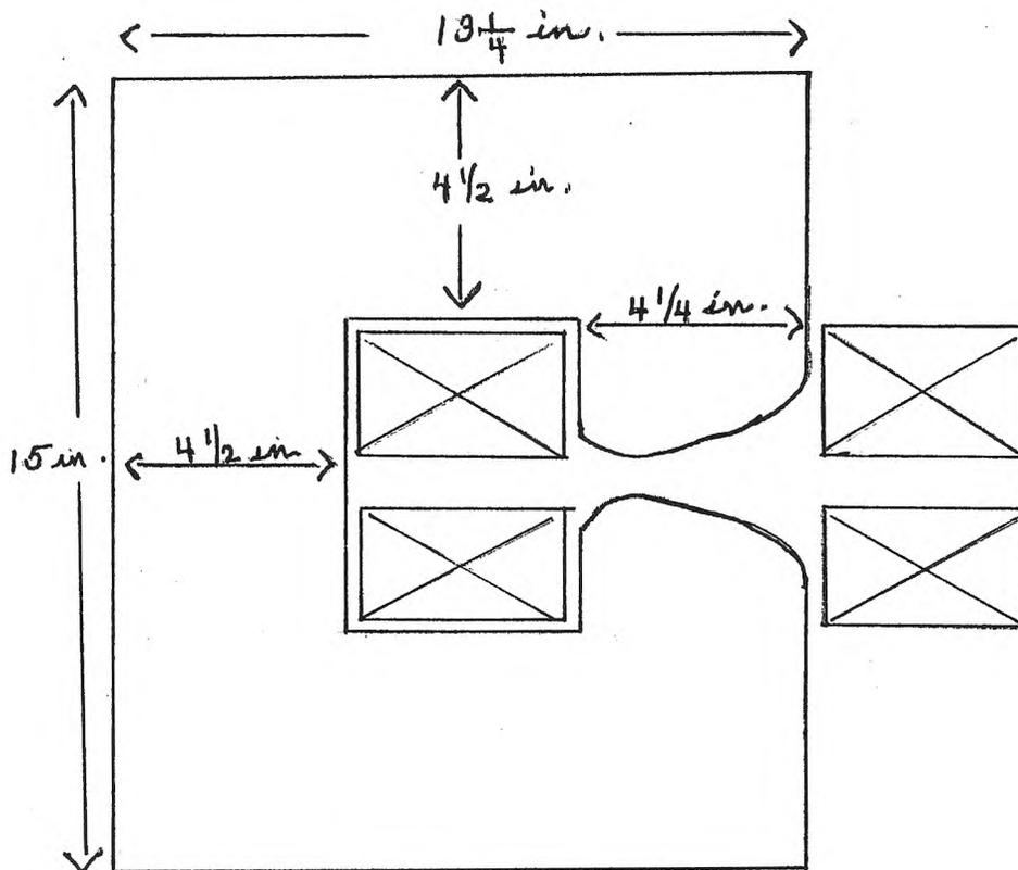
This leads to a coil cross-section about 4 inches by 2-1/4 inches. Scaled from the A.G.S. the magnet's minimum gap is just a little over 3/4 inch and the pole tip width is about 4-1/4 inch. Other magnet dimensions might be as shown in the figure. Approximate weights are, then, about 6000 tons of steel and about 1400 tons of copper.
