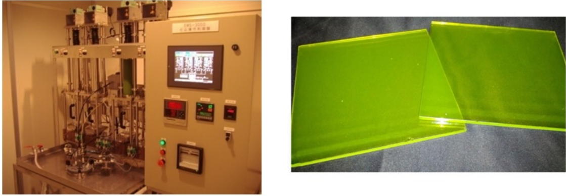
Figure 22: Left: Self-production machine for nuclear emulsion gel. Right: NIT device coated onto a glass base.
