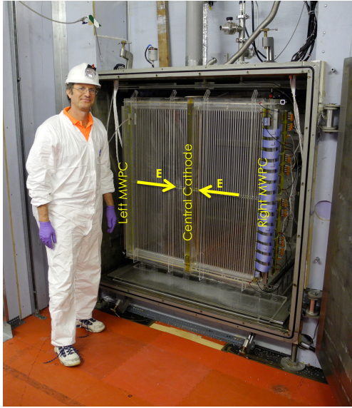
Figure 3: The DRIFT-II detector in the Boulby Mine.
