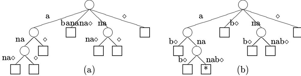
Figure 1: (a) A suffix tree for the string  $\text{banana}\diamond$ . (b) A suffix tree for  $\text{ananab}\diamond$ , or, equivalently, a “prefix tree” for  $\diamond\text{banana}$ .
