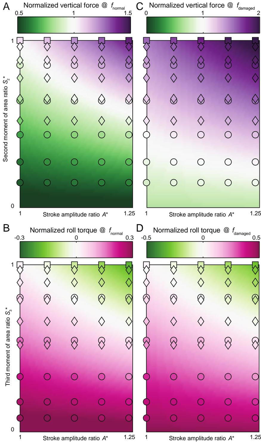
**Figure S3.** Aerodynamic forces and torques produced by the robotic fruit fly with a right wing with variable stroke amplitudes and variable damage (the left wing was left intact and flapped with a constant stroke amplitude). All data points were color coded with vertical force (A,C) or roll torque (B,D) according to the color-bar above each panel.
