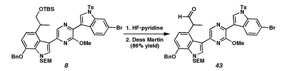
Aldehyde 43. To a Falcon tube containing a THF (5 mL) solution of bis-indole 8 (70 mg, 0.07 mmol) at 0 °C, was added HF•pyridine (800  $\mu$ L) in a dropwise fashion. The reaction mixture was stirred at 0 °C for 1.5 h until the reaction was judged complete by TLC. After dilution of the mixture with ether (10 mL), saturated aqueous sodium bicarbonate (10 mL) was added in a dropwise manner at 0 °C. The layers were separated and the organic portion was
