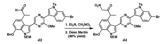
**Ketone 44.** To aldehyde **43** (20 mg, 0.023 mmol) in nitromethane (1 mL) was added triethylamine (75  $\mu$ L, 0.54 mmol). The reaction mixture was stirred at 23 °C for 15 h. The excess nitromethane was removed by evaporation under reduced pressure to afford the crude nitroaldol product which was used without further purification.
