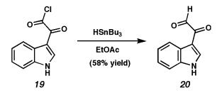
**Ketoaldehyde 20.** To a suspension of **19** (22.0 g, 106 mmol) in EtOAc (106 mL) at 0 °C, was added a solution of tributyltin hydride (28.5 mL, 106 mmol) in EtOAc (158 mL). The reaction mixture was stirred at 0 °C for 30 min, warmed to 23 °C, then stirred for an additional 15 h. Hexane (150 mL) was added and the resulting yellow powder was collected by filtration. Washing with copious amounts of hexanes (1 L) and drying under vacuum, gave ketoaldehyde **20**
