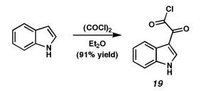
Acid chloride 19. To a solution of indole (20.0 g, 171 mmol) in anhydrous diethyl ether (340 mL) at 0 °C, oxalyl chloride (17.3 mL, 198 mmol) was added dropwise over 30 min. The reaction mixture was stirred at 0 °C for 3 h, then allowed to warm to 23 °C over 1 h. The resulting yellow crystals were collected by filtration, washed with cold anhydrous ether (100 mL), and dried under vacuum to yield **19** (32.52 g, 92% yield) which was used without further purification.
