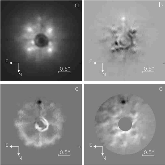
**Fig. 3.** Coronagraphic images of the binary star HD 222493 obtained with 600 frames lasting 60 ms each and a  $0.63''$  mask. The companion is already visible on the direct integration of frames **a**) and is enhanced on the subtraction map **b**). Lower images **c**), **d**) show the subtraction result using dark-speckle process with a constant threshold of 100 ADU **c**) and a radial threshold **d**), see Sect. 4. The companion now appears as a dark feature with an improved  $SNR$
