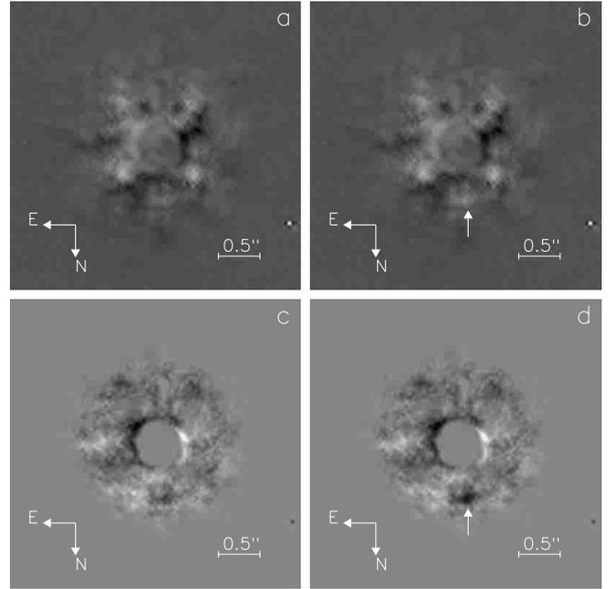
**Fig. 6.** Coronagraphic subtracted images of HD 192876 for direct integration of frames **a,b**) and with a dark-speckle analysis **c,d**). A faint companion ( $\Delta m_k = 6$ , arrow) is added to the map **b,d**) to assess the detection threshold. The  $SNR$  is 1.8 with a direct integration and improves to 4.8 owing to the dark-speckle process
