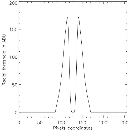
**Fig. 1.** An example of radial threshold obtained for the star HD 222493. A mask is used to select the region of interest: pixel 86 to 170
