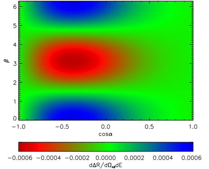
FIG. 2: Contour plot of the differential event rate, Eq. (12), in units of events/kg/day/keV/sr as a function of  $\cos\alpha$ , where  $\alpha$  is the polar angle, and the azimuthal angle  $\beta$ , for fixed recoil energy  $E = 30$  keV. We take the angle between the polarization and the detector velocity through the Galactic halo to be  $\vartheta = 90^\circ$ . We also take  $G = (100 \text{ GeV})^{-2}$ , and  $m_\chi = 100$  GeV.
