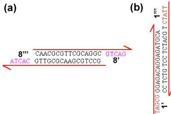
**Figure S2.** Double-stranded DNA bridges used in Figures 2 and 3. Schematic drawings of (a) horizontal, (x-direction), and (b) vertical (y-direction) bridges. Each bridge is composed of two strands with the two sticky-ends at the ends of dsDNA molecules. The complementary sticky-end of n is n' and of n'' is n'''.
