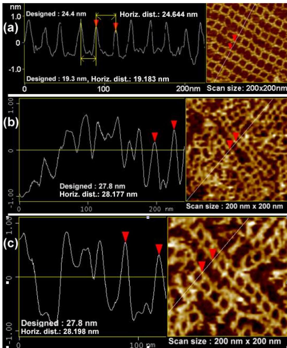
**Fig. S7.** Section measurements of Nanotracks + double stranded DNA bridges. Section profile AFM images of (a) nanotracks with the short dsDNA bridges. The measured distance between nanotracks is  $\sim 24.6$  nm, matching the designed distance, 24.4 nm. (b) and (c) are two examples of section profiles of nanotracks with the long dsDNA bridges. Both data are in good agreement with designed structures with less than  $\pm 1$  nm differences.
