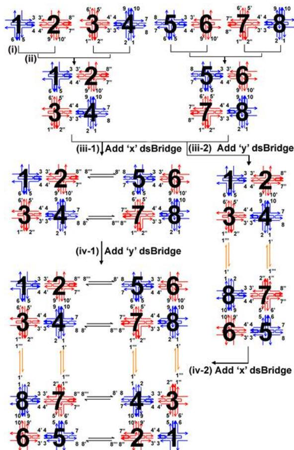
**Figure S3.** Four-step self-organization of the finite-size superstructures composed of  $2 \times 2$  NAs and dsDNA nanobridges.
