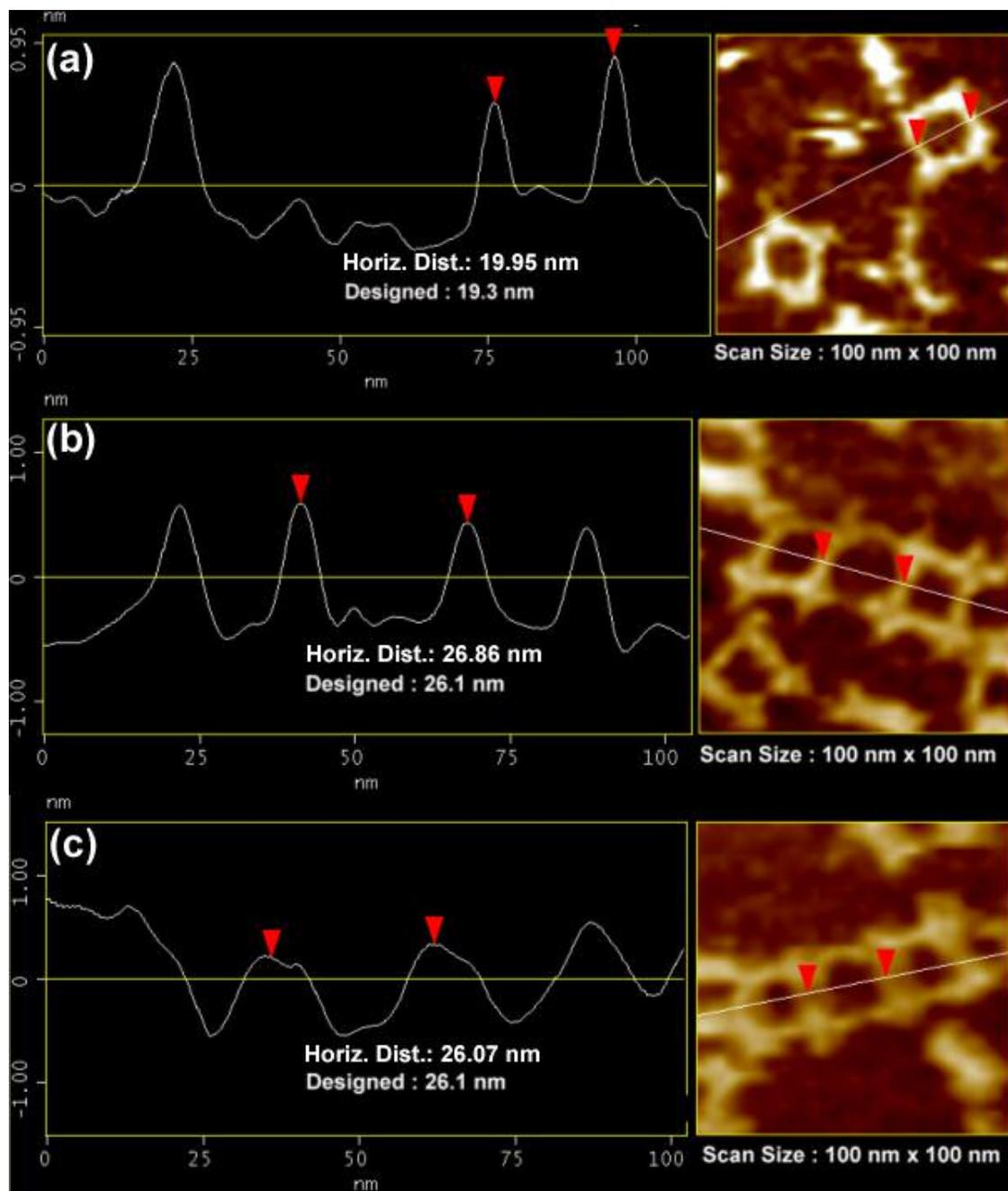
**Figure S4.** Section measurement of  $2 \times 2$  NA + dsDNA bridges. Section profile distance measurements of (a)  $2 \times 2$  NA, (b)  $2 \times 2$  NA with horizontal, and (c)  $2 \times 2$  NM with vertical dsDNA bridges. All experimental distance measurements were in excellent agreement with designed structures with less than 5% ( $\pm 1.0$  nm) deviation.
