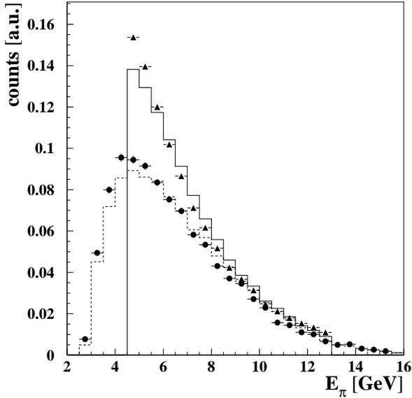
**Fig. 3.** Comparison between the measured and simulated pion energy spectra. Filled circles (triangles) are the neutral (charged) pion measurements. The histograms are the simulated spectra for neutral (dashed line) and charged (full line) pions. All spectra have been normalized to unit area.
