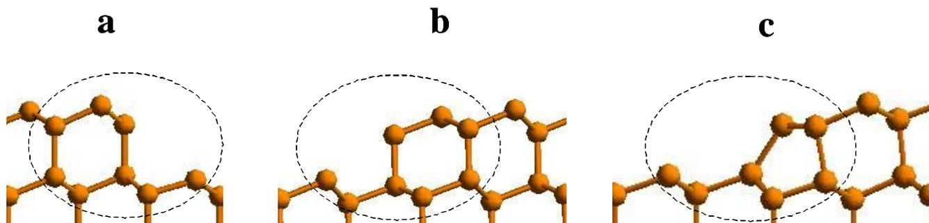
**Figure S-2.** Structures of the Si(111) surface step edges: (a)  $\langle 11\bar{2} \rangle$  edge, (b) unreconstructed  $\langle \bar{1}\bar{1}2 \rangle$  edge, and (c) reconstructed  $\langle \bar{1}\bar{1}2 \rangle$  edge.
