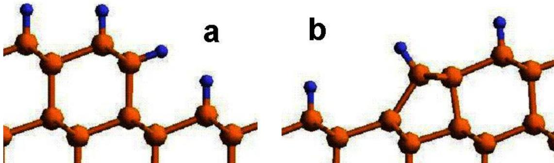
**Figure S-5.**  $\langle 11\bar{2} \rangle$  (a) and  $\langle \bar{1}\bar{1}2 \rangle$  (b) step edges for the Si(111)-H surface. Note that the  $\langle \bar{1}\bar{1}2 \rangle$  structure (b) has reconstructed in order to have its substituents perpendicular to the edge surface and to lower its energy. <sup>6</sup>
