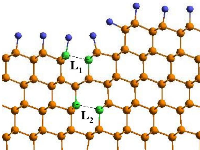
**Figure S-4.** Illustration of overstretched Si-Si bonds in the chlorinated  $\langle 11\bar{2} \rangle$  step edge. The blue atoms are Cl, the orange atoms are bulk Si and the green atoms are Si with overstretched bonds. In the optimum structure,  $L_1 = 2.82 \text{ \AA}$  and  $L_2 = 2.87 \text{ \AA}$  (compare to  $L_{\text{bulk}} = 2.36 \text{ \AA}$ )
