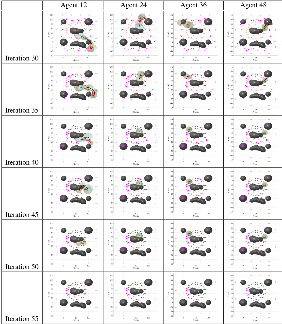
Figure 8. Multiple iterations of the entire Multi-Agent SE-SCP algorithm for agents 12, 24, 36, and 48 are shown. The location of the agents are shown using magenta dots.
