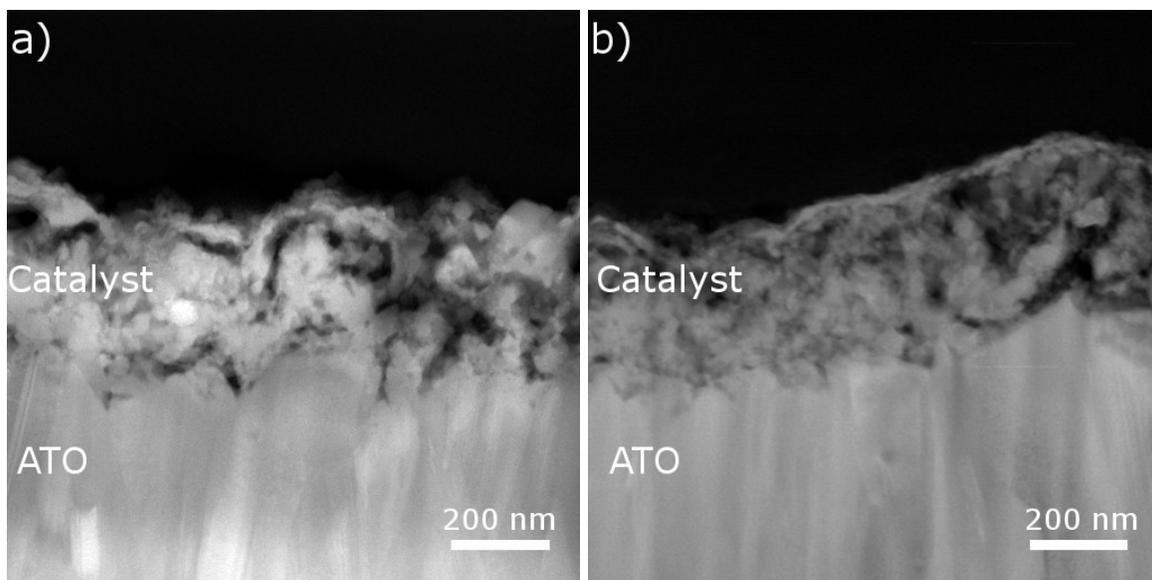
**Figure S9.** High-angle annular dark-field (HAADF) images of (a)  $\text{Ni}_{0.5}\text{Mn}_{0.5}\text{Sb}_{1.7}\text{O}_y$  before electrochemical operation, and (b)  $\text{Ni}_{0.5}\text{Mn}_{0.5}\text{Sb}_{1.7}\text{O}_y$  after chronopotentiometry for 144 h at  $10 \text{ mA cm}^{-2}$ . The lower portion of the image was identified as the ATO support, and a porous film
