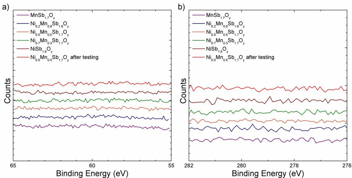
**Figure S12.** High-resolution XPS data of as-synthesized  $\text{Ni}_x\text{Mn}_{1-x}\text{Sb}_{1.6-1.8}\text{O}_y$  and  $\text{Ni}_{0.5}\text{Mn}_{0.5}\text{Sb}_{1.7}\text{O}_y$  after chronopotentiometry for 144 h at  $10 \text{ mA cm}^{-2}$ . The spectral regions are: (a) Ir 4f and (b) Ru 3d. No Ir or Ru was detected on the surface by XPS.
