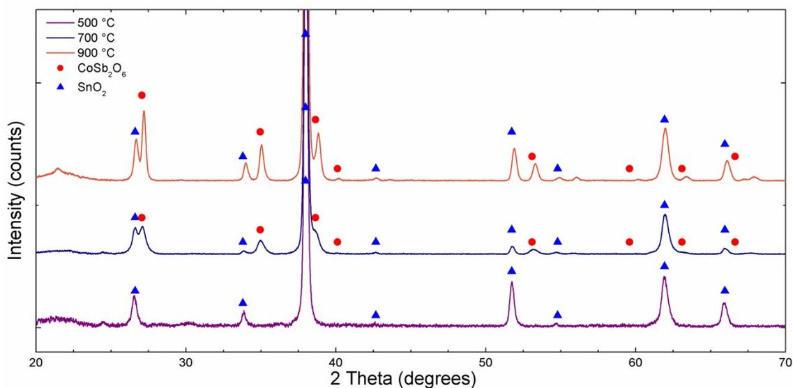
**Figure S14.** X-ray diffraction of  $\text{Ni}_{0.5}\text{Mn}_{0.5}\text{Sb}_{1.7}\text{O}_y$  films annealed at 500 °C, 700 °C, and 900 °C. Reference patterns are  $\text{SnO}_2$  (red circles) and  $\text{CoSb}_2\text{O}_6$  (blue triangles).
