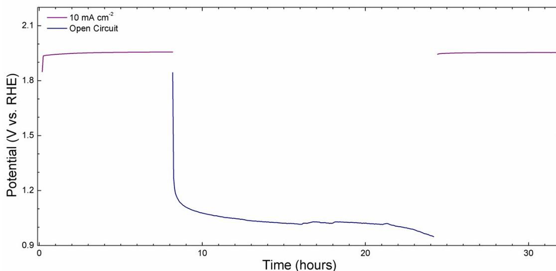
**Figure S5.** Potential of a Ni<sub>0.5</sub>Mn<sub>0.5</sub>Sb<sub>1.7</sub>O<sub>y</sub> electrode being held at 10 mA cm<sup>-2</sup> for 8 h, followed by 16 h at open circuit and subsequently being held at 10 mA cm<sup>-2</sup> for 8 h.
