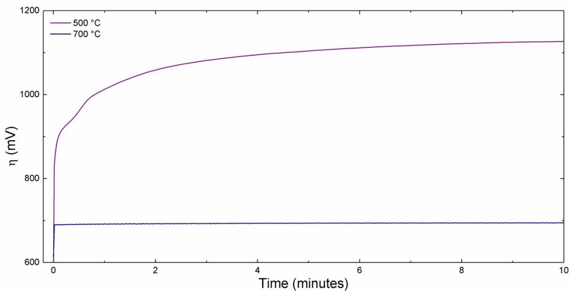
**Figure S13.** Chronopotentiometry at  $10 \text{ mA cm}^{-2}$  of  $\text{Ni}_{0.5}\text{Mn}_{0.5}\text{Sb}_{1.7}\text{O}_y$  films annealed at  $500 \text{ }^\circ\text{C}$  and  $700 \text{ }^\circ\text{C}$ .
