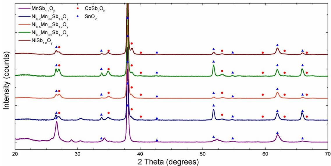
**Figure S1.** X-ray diffraction pattern for  $\text{Ni}_x\text{Mn}_{1-x}\text{Sb}_{1.6-1.8}\text{O}_y$  thin films on an ATO substrate. The peaks were indexed to reference patterns of  $\text{SnO}_2$  and  $\text{CoSb}_2\text{O}_6$ .<sup>2,3</sup>
