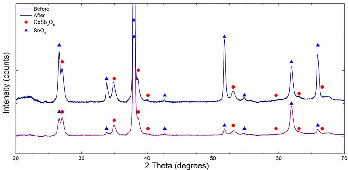
**Figure S8.** Diffraction pattern of  $\text{Ni}_{0.5}\text{Mn}_{0.5}\text{Sb}_{1.7}\text{O}_y$  before and after chronopotentiometry for 144 h at  $10 \text{ mA cm}^{-2}$  of geometric area. The peaks were indexed to reference patterns of  $\text{SnO}_2$  and  $\text{CoSb}_2\text{O}_6$ .<sup>2,3</sup>
