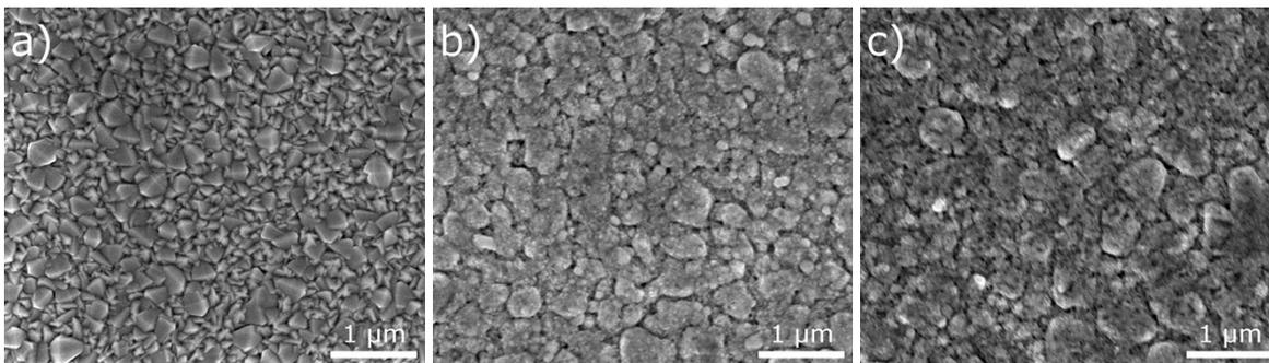
**Figure S10.** SEM images of (a) ATO substrate, (b) Ni<sub>0.5</sub>Mn<sub>0.5</sub>Sb<sub>1.7</sub>O<sub>y</sub> before electrochemical operation, and (c) Ni<sub>0.5</sub>Mn<sub>0.5</sub>Sb<sub>1.7</sub>O<sub>y</sub> after chronopotentiometry for 144 h at 10 mA cm<sup>-2</sup>.
