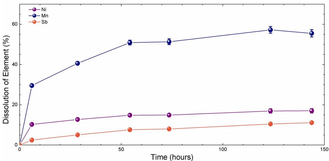
**Figure S7.** Cumulative dissolution of a Ni<sub>0.5</sub>Mn<sub>0.5</sub>Sb<sub>1.7</sub>O<sub>y</sub> electrode during chronopotentiometry at 10 mA cm<sup>-2</sup>. The active electrode geometric area was 0.920 cm<sup>2</sup>.
