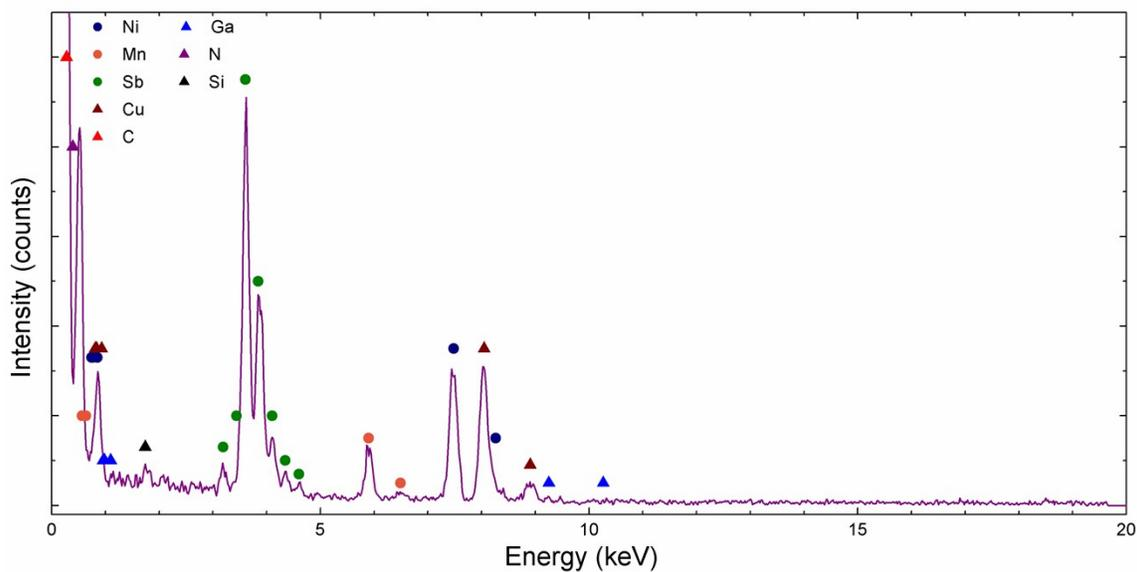
**Figure S11.** STEM-EDS data of as-synthesized Ni<sub>0.5</sub>Mn<sub>0.5</sub>Sb<sub>1.7</sub>O<sub>y</sub> showing that only Ni, Mn, Sb were detectable in the film. Cu, C, Ga, N, and Si are from the TEM grid and TEM sample preparation.
